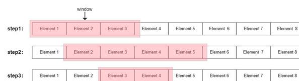
Figure 17. Schematic diagram of sliding window algorithm.
