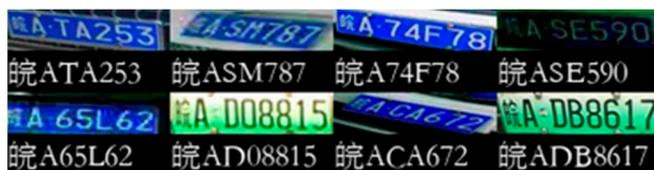
**Figure 7.** The recognition results of the LPRNet model.
