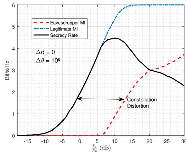
Figure 7. Achievable SR of a malicious eavesdropper and legitimate user. MI between the legitimate user and the eavesdropper. Both users positioned in the far field with  $\Delta\theta = 10^\circ$ .
