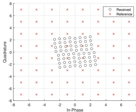
**Figure 9.** I-Q diagram of the 64-QAM constellation received by the eavesdropper when  $\Delta d = 25\lambda$  in the near field.
