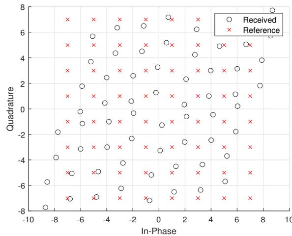
Figure 6. I-Q diagram of the 64-QAM constellation received by the eavesdropper when  $\Delta\theta = 5^\circ$ .
