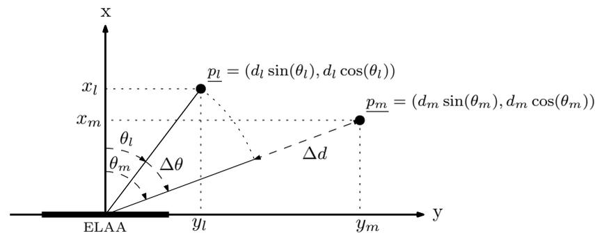
Figure 2. Top view of the considered communication scenario with an ELAA transmitting to a legitimate user and a malicious eavesdropper.
