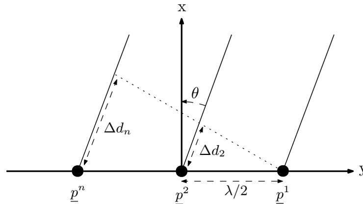
Figure 3. Considered ULA geometry with signals being transmitted with an angle-of-departure  $\theta$ .
