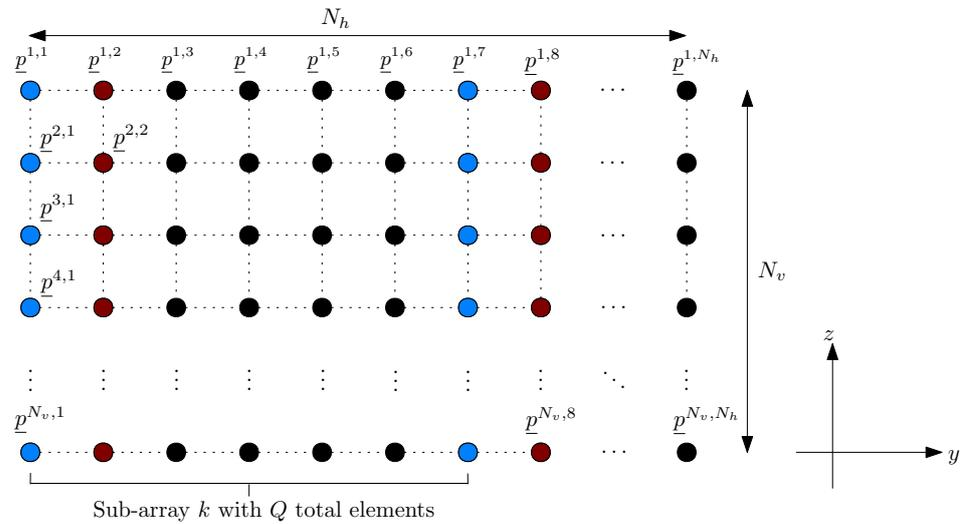
Figure 1. Considered ELAA deployed on the YZ plane.
