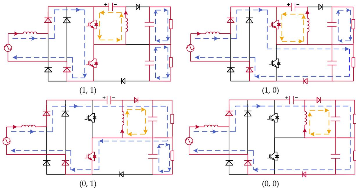
Figure 2. All the operating modes and the corresponding current flowing paths of the rectifier.
