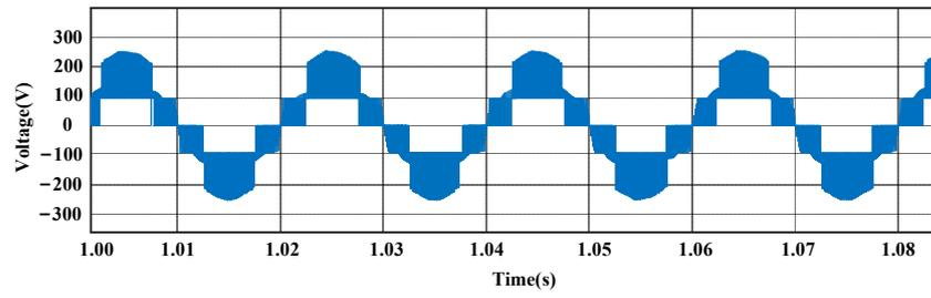
Figure 12. The input voltage of the single-phase diode bridge rectifier in boost mode.
