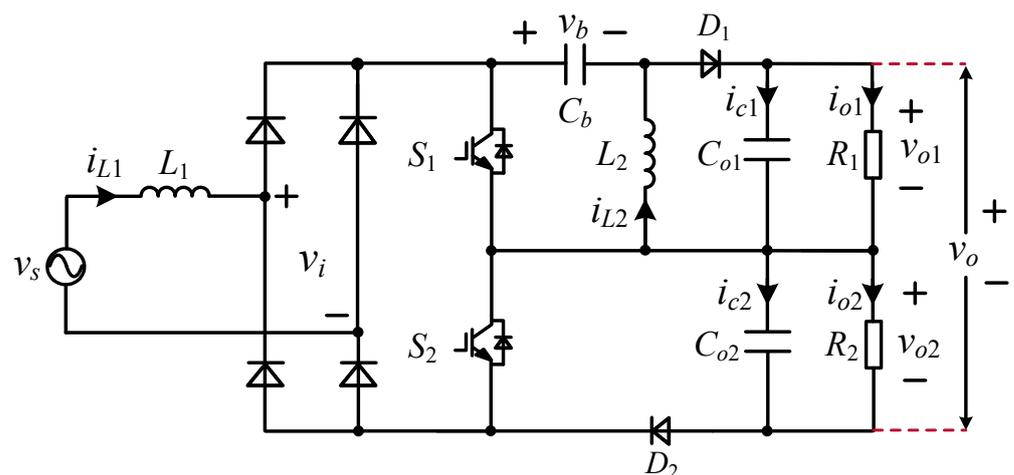
Figure 1. The proposed unidirectional hybrid single-phase rectifier topology.
