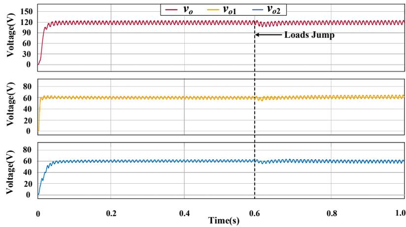
Figure 14. The DC capacitor voltages of the single-phase diode bridge rectifier in buck mode.
