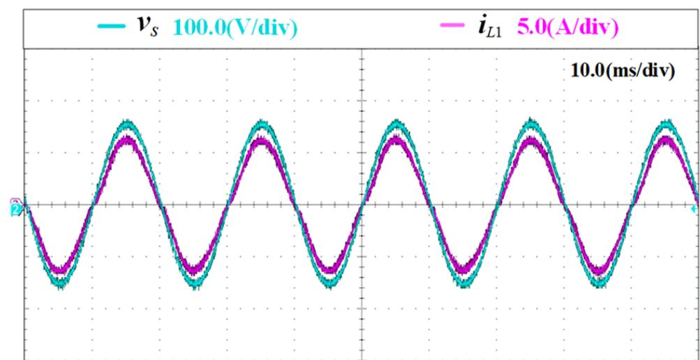
Figure 16. The power supply voltage  $v_s$  and input current  $i_{L1}$  experimental waveforms.
