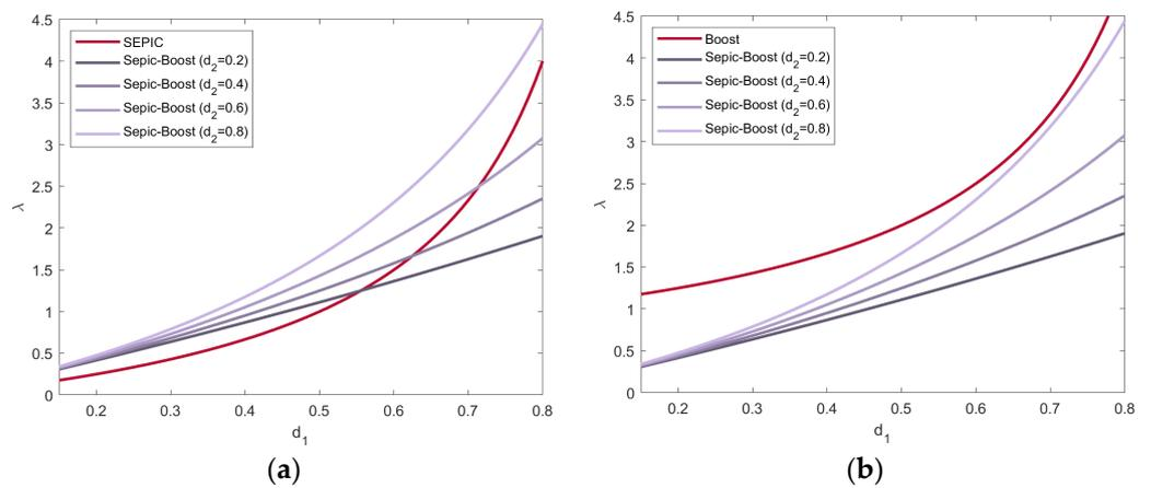
Figure 5. Comparison of voltage transfer ratio  $\lambda$  of the proposed rectifier: (a) with SEPIC rectifier; (b) with boost rectifier.
