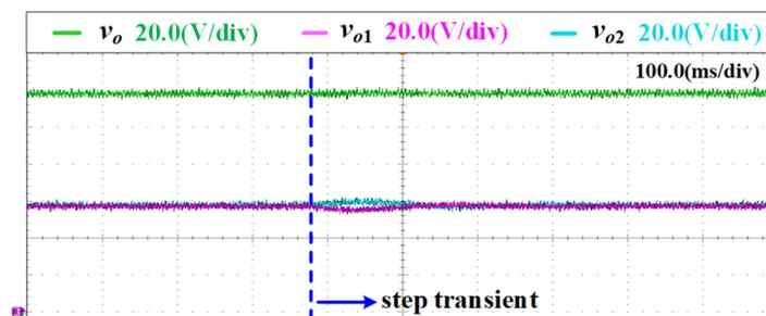
Figure 20. The experimental results of the DC-link voltage  $v_o$  and the DC capacitor voltages  $v_{o1}$  and  $v_{o2}$  in buck mode.
