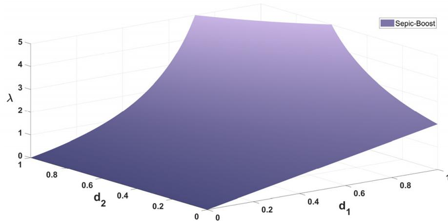
Figure 4. Voltage transfer ratio of the proposed rectifier  $\lambda$ .
