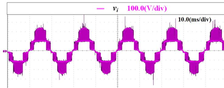
Figure 18. The input voltage of the single-phase diode bridge rectifier experimental waveforms.
