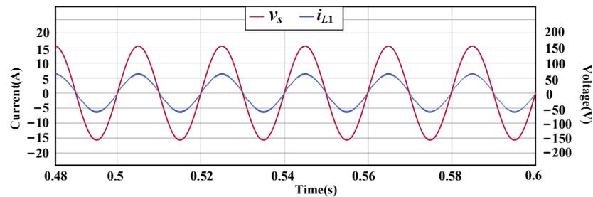
**Figure 10.** The power supply voltage  $v_s$  and input current  $i_{L1}$  simulation waveforms.
