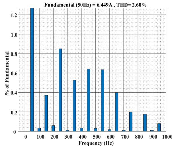
**Figure 11.** The THD analysis of input current  $i_{L1}$ .
