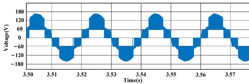
Figure 15. The input voltage of the single-phase diode bridge rectifier in buck mode.
