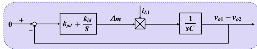
Figure 8. The basic control structure of the DC capacitor voltages loop.
