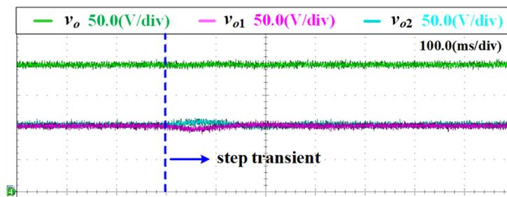
Figure 19. The experimental results of the DC-link voltage  $v_o$  and the DC capacitor voltages  $v_{o1}$  and  $v_{o2}$  in boost mode.
