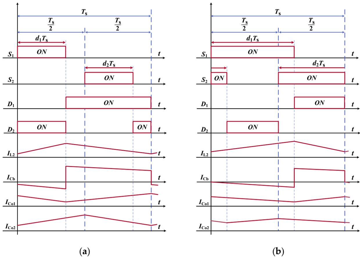
Figure 3. Main waveforms of the proposed rectifier: (a)  $0 < d < 0.5$ ; (b)  $0.5 \leq d < 1$ .
