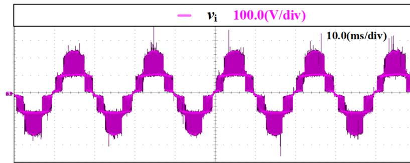
**Figure 21.** The experimental waveforms of the input voltage of the single-phase diode bridge rectifier in buck mode.
