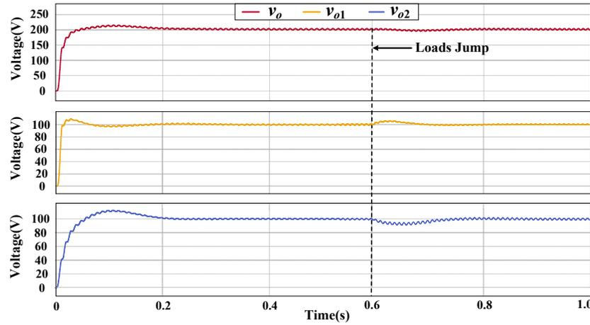
Figure 13. The DC capacitor voltages of the single-phase diode bridge rectifier in boost mode.
