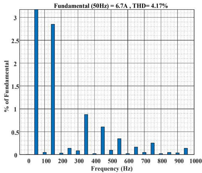
Figure 17. The input current  $i_{L1}$  harmonic spectrum.
