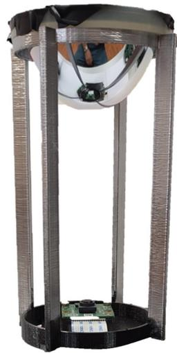
**Figure 7.** The catadioptric system of the NEXUS 2 robot.
