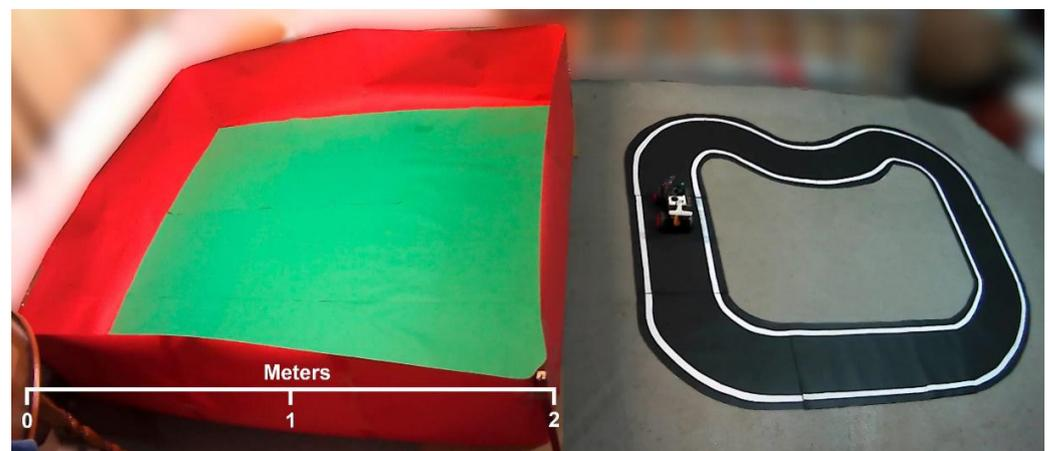
**Figure 1.** Components of the complete working environment. Depending on the required task, the driving circuit will be placed either in the chroma scenario (**left**) or in the target scenario (**right**). The driving circuit can be placed in either stage when needed.
