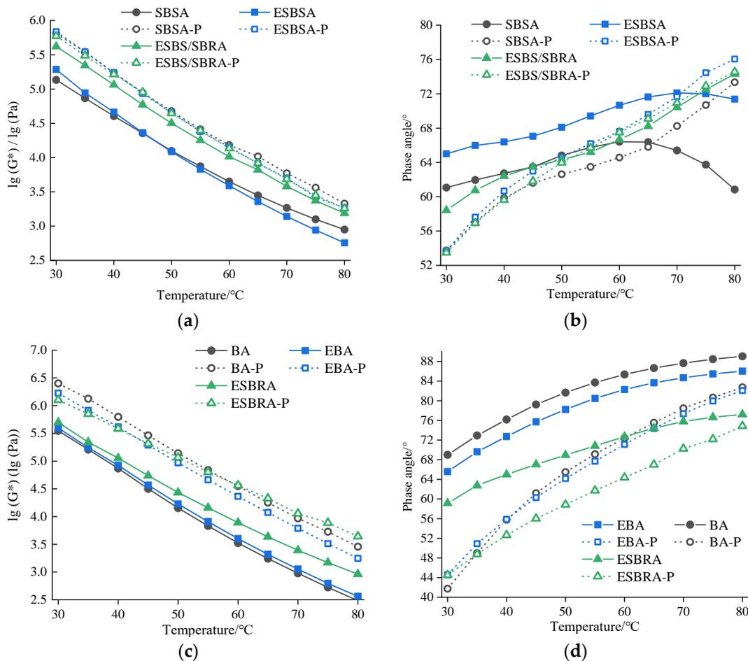
**Figure 6.** Temperature sweep results of emulsified asphalt residues before and after aging. (a) Complex modulus of SBS and ESBS. (b) Phase angle of SBS and ESBS. (c) Complex modulus of BA and SBR. (d) Phase angle of BA and SBR.
