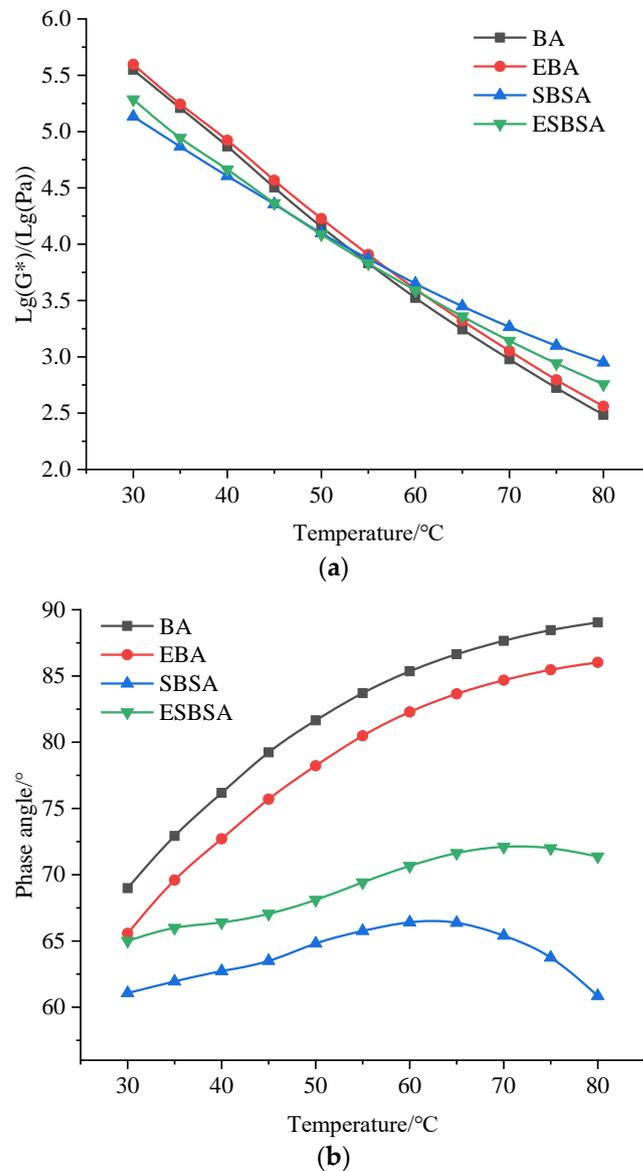
Figure 4. Temperature sweep test results of emulsified asphalt. (a) Complex modulus. (b) Phase angle.
