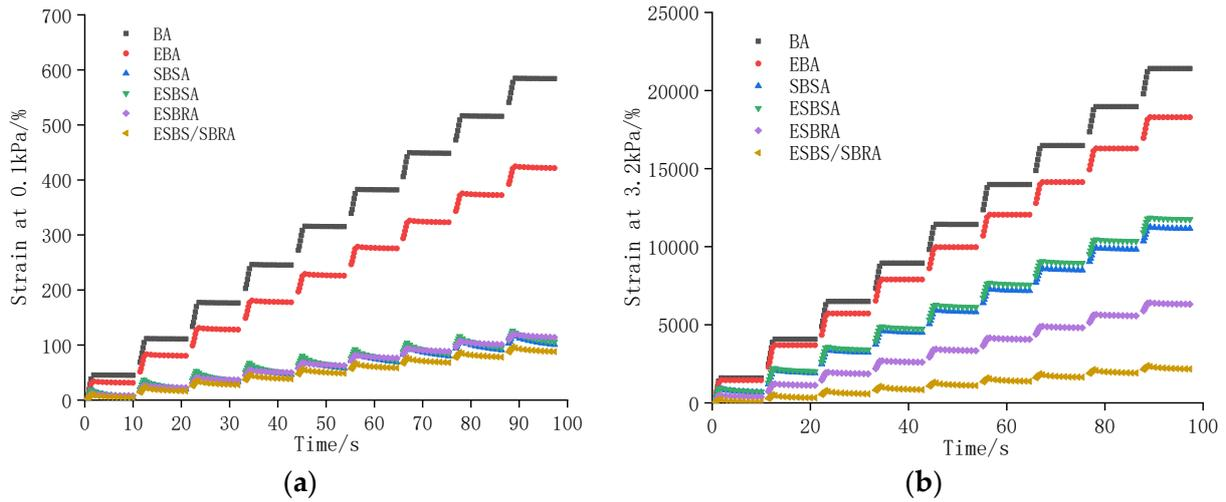
Figure 7. Results of MSCR test. (a) Stress @0.1 kPa. (b) Stress @3.2 kPa.
