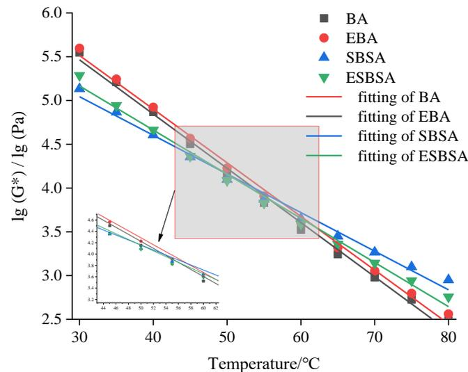
**Figure 5.** Fitting curve of asphalt composite modulus-temperature before and after emulsification.
