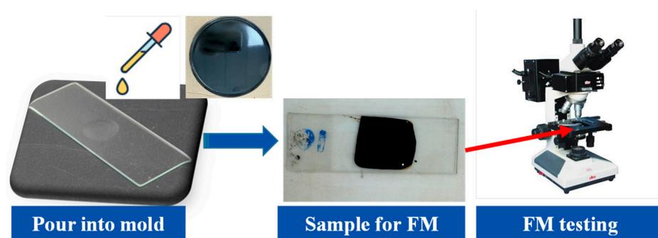
**Figure 3.** Fluorescence microscopy of asphalt.
