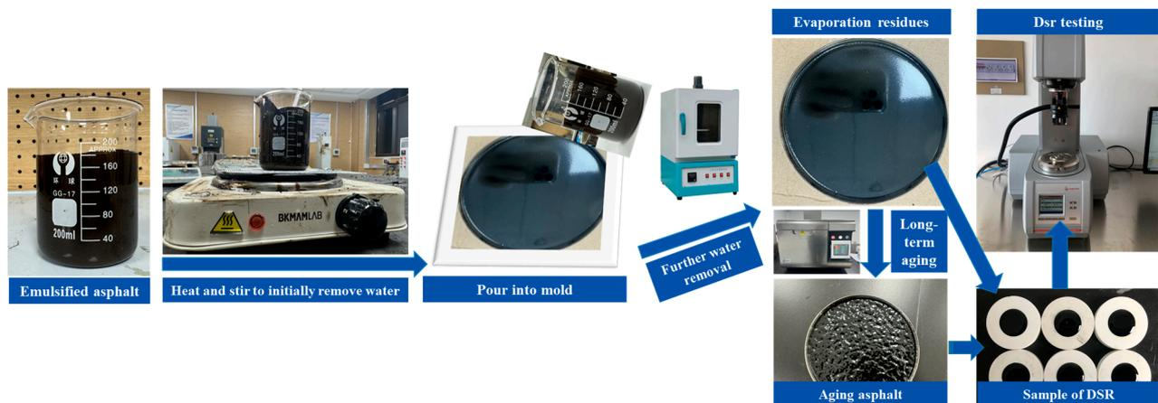
**Figure 2.** Diagram of emulsified asphalt residue DSR test samples.
