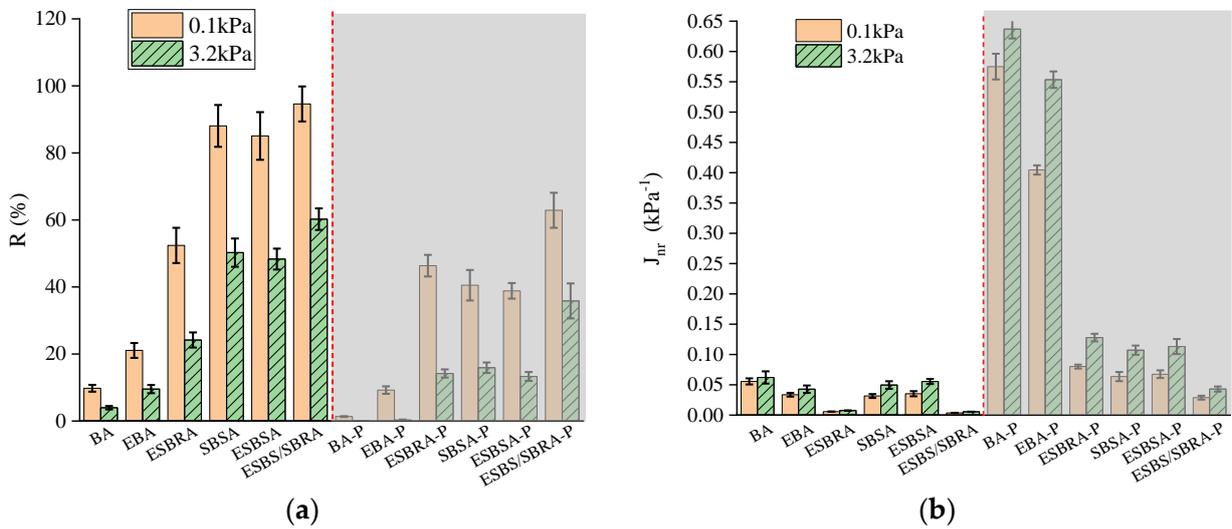
Figure 8. Results of high-temperature performance evaluation based on MSCR test. (a) R. (b)  $J_{nr}$ .
