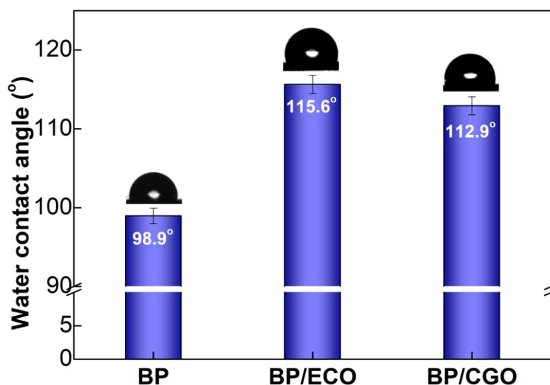
**Figure 3.** Water contact angles of control and plant-oil-modified bleached Kraft papers.
