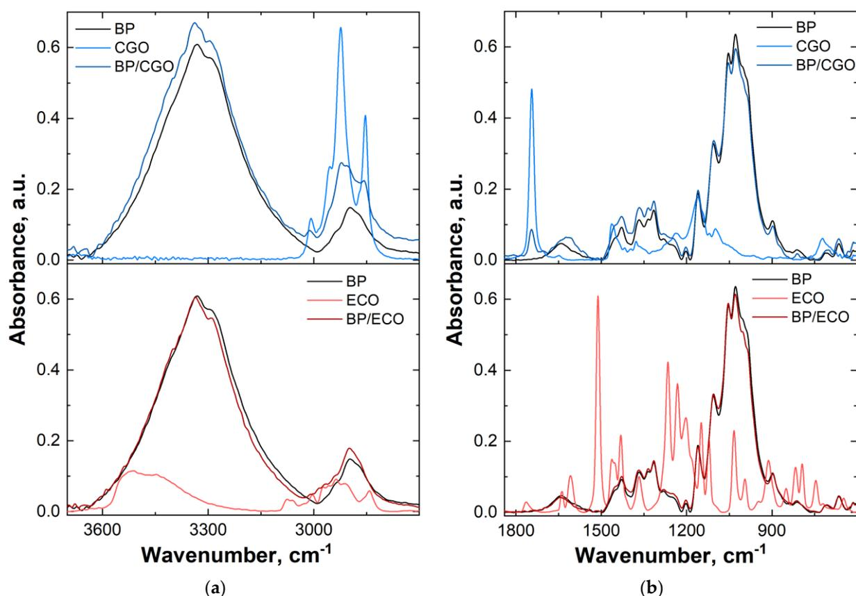
**Figure 1.** Infrared spectra of control and plant-oil-modified Kraft paper in the 3700–2700  $\text{cm}^{-1}$  region (a) and 1800–600  $\text{cm}^{-1}$  region (b).
