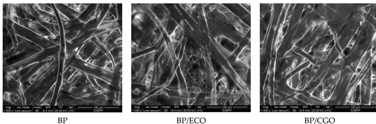
**Figure 2.** SEM images of the control and plant-oil-modified bleached Kraft paper.
