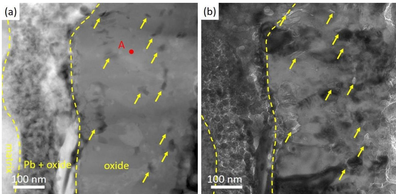
**Figure 5.** HAADF and bright field images of the oxide layer of as-received specimen after Pb corrosion. (a,b) HAADF and bright field images of the same spot, with arrows indicating the voids located between oxides grains. The bright field image was taken at 1000 nm under focus.
