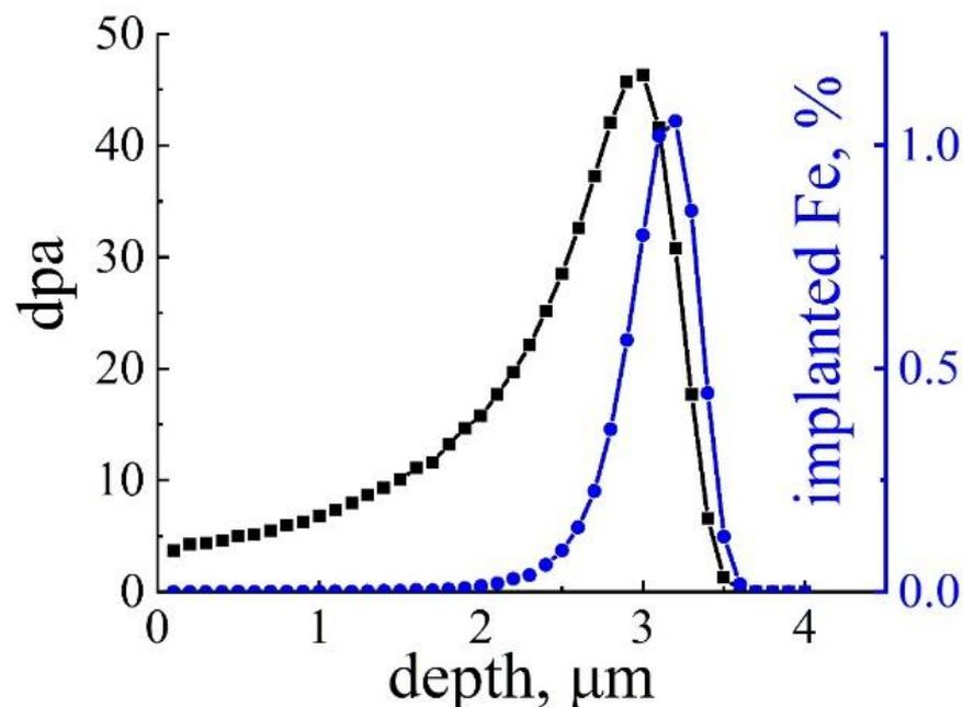
**Figure 1.** Damage and injected ions profile of 19.6 MeV Fe ion irradiation to total fluence of  $5 \times 10^{16}$  ions/cm<sup>2</sup> calculated by SRIM 2013.
