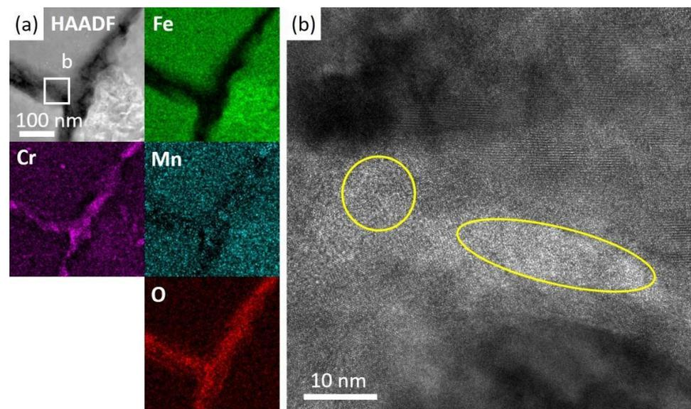
**Figure 11.** TEM and EDS images of grain boundaries in the irradiated specimen after corrosion. (a) Oxides of Cr and a small amount of Mn at the grain boundaries in the irradiated specimen after corrosion. (b) High-resolution image of the oxides. Some of the oxides had a crystalline structure while others were amorphous, indicated by circles.
