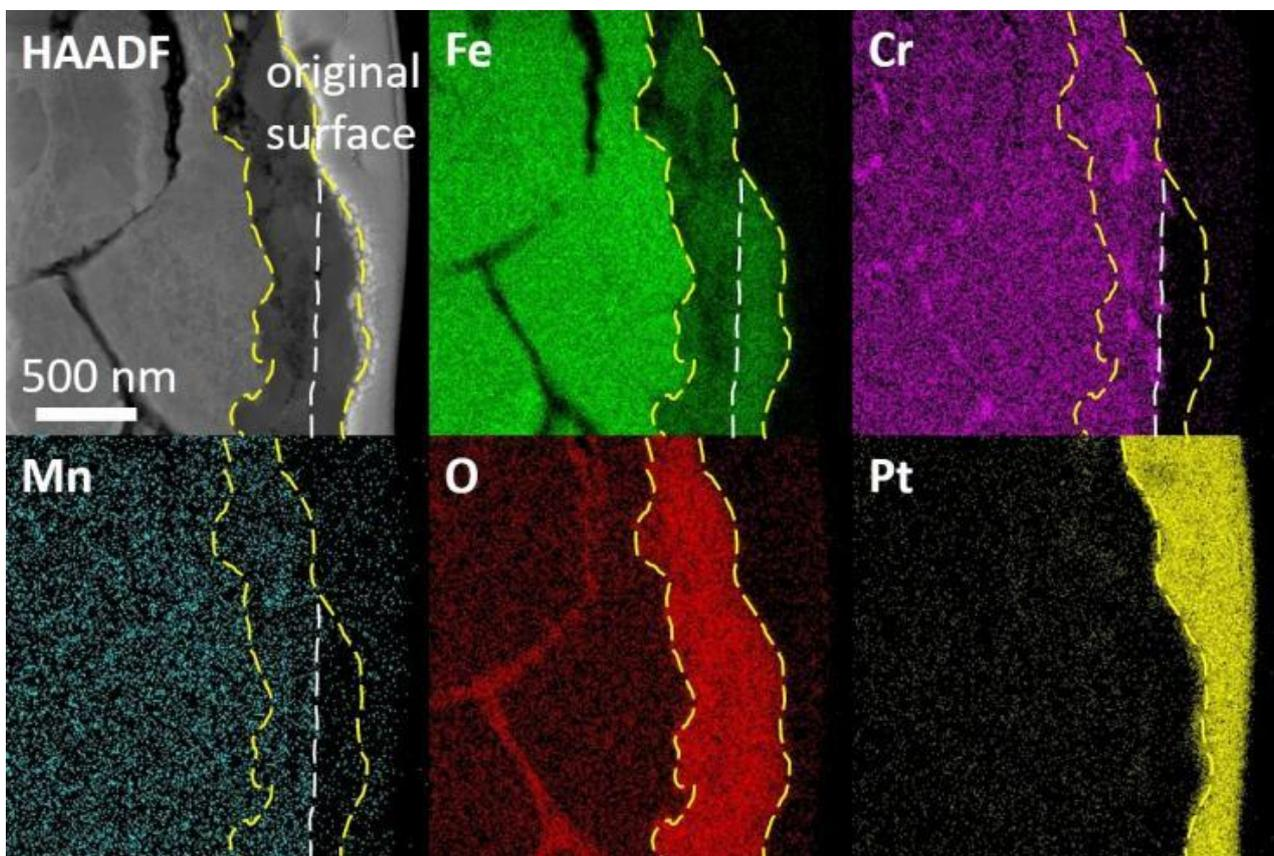
**Figure 8.** TEM and EDS images of the bi-layer oxide scale in the irradiated specimen after Pb corrosion. The original surface, marked by dash line, divided the outer layer and the inner layer.
