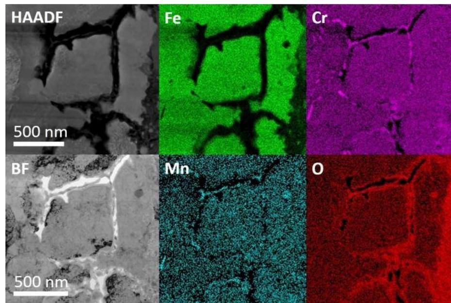
**Figure 10.** TEM and EDS images of the grain boundary oxidation with mainly Cr and Mn oxides beneath the oxide layer in the irradiated specimen after corrosion.
