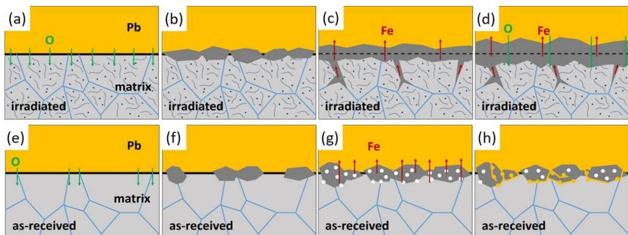
**Figure 12.** Schematic diagram for the corrosion process of the irradiated specimen in (a–d) and the as-received specimen in (e–h).
