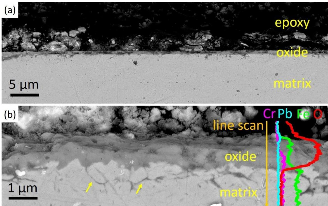
**Figure 7.** SEM cross-sectional images of the irradiated specimen after Pb corrosion at 550 °C for 1h. (a) Uniform oxide layer formed in the surface of steel matrix and no Pb penetration was observed. (b) A zoomed-in image of the oxide layer and its EDS line scan results. Oxidation along grain boundaries was observed in some areas indicated by arrows.
