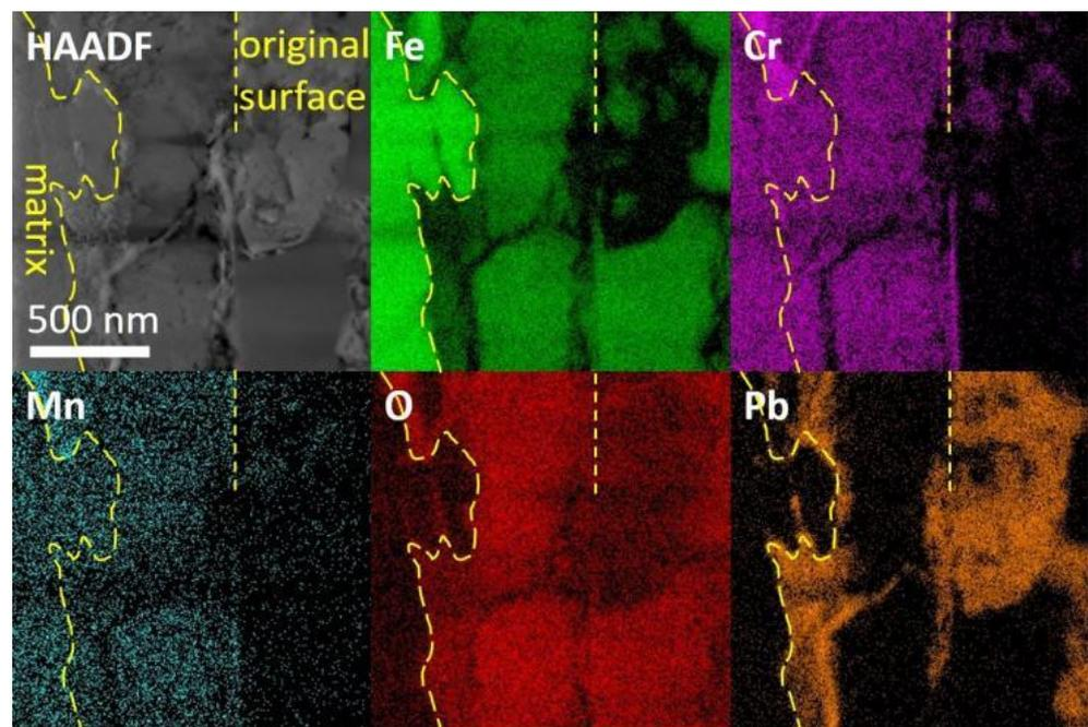
**Figure 4.** TEM and EDS images of the oxide layer in the as-received specimen after Pb corrosion. Fe and Cr oxides formed beneath the original surface. Pb was observed between oxides and steel matrix.
