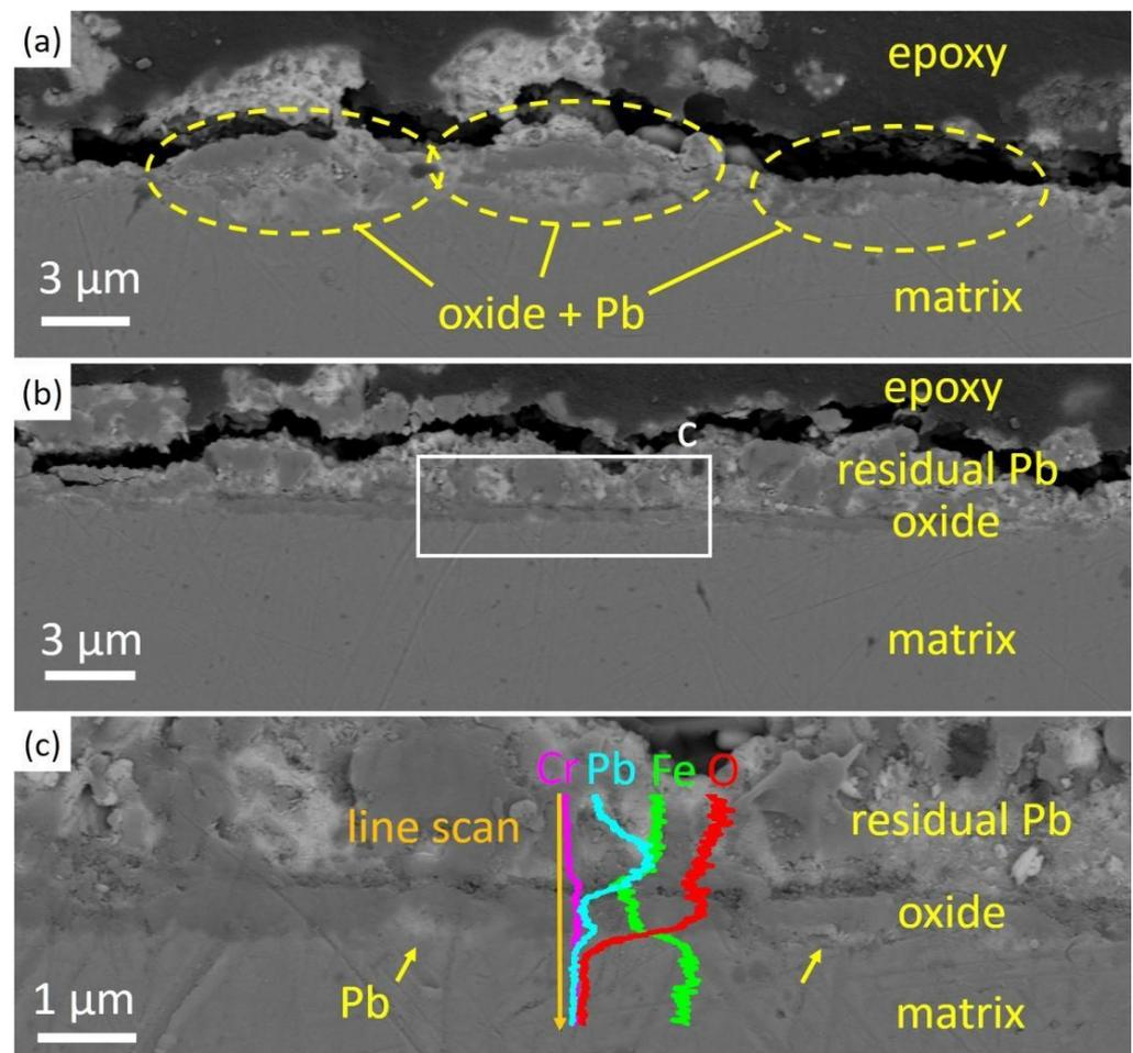
**Figure 3.** SEM cross-sectional images of the as-received specimen after Pb corrosion at 550 °C for 1 h. (a,b) Discontinuous oxides without protectiveness to the steel matrix. (c) A zoomed-in image of oxide layer. Pb penetration into the oxides are indicated with yellow arrows. EDS line scan results across the oxides show the presence of Pb inside the oxide layer.
