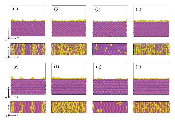
**Figure 3.** Snapshots of relaxed structures of eight SiC(0001)/Al models colored using the Wigner–Seitz defect analysis. Al-atoms offsetting the original FCC lattice space are colored yellow, C-atoms are colored red, and Si-atoms are colored blue. (a) SiC(0001)-Si/Al(001), (b) SiC(0001)-Si/Al(110), (c) SiC(0001)-Si/Al(111), (d) SiC(0001)-Si/Al(112), (e) SiC(0001)-C/Al(001), (f) SiC(0001)-C/Al(110), (g) SiC(0001)-C/Al(111), (h) SiC(0001)-C/Al(112).
