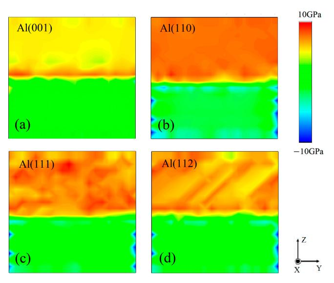
**Figure 5.** Stress distribution before cracks' nucleation of four SiC(0001)-Si/Al interface systems: (a) SiC(0001)-Si/Al(001), (b) SiC(0001)-Si/Al(110), (c) SiC(0001)-Si/Al(111), (d) SiC(0001)-Si/Al(112).
