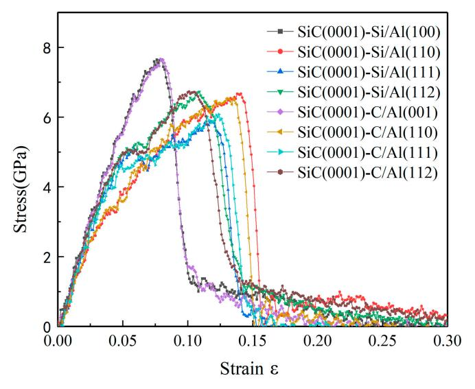
Figure 2. Engineering stress-strain curves of eight interface model systems under tensile loading.
