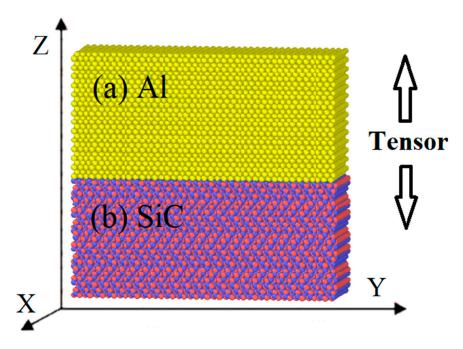
**Figure 1.** SiC(0001)-Si/Al(001) tensile model structure given as an example: (**a**) Al, (**b**) SiC. Al-atoms are colored yellow, C-atoms are colored red, and Si-atoms are colored blue.
