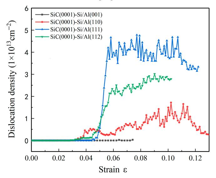
Figure 6. Dislocation density of the four SiC(0001)-Si/Al models during the tensile process.
