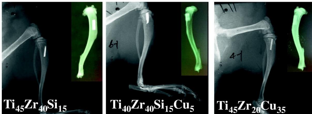
**Figure 20.** X-ray image of the Sprague-Dawley rat with MG tibia implants of the  $\text{Ti}_{45}\text{Zr}_{40}\text{Si}_{15}$ ,  $\text{Ti}_{40}\text{Zr}_{40}\text{Si}_{15}\text{Cu}_5$ , and  $\text{Ti}_{45}\text{Zr}_{20}\text{Cu}_{35}$  alloys. The main images were taken immediately after implantation, the insets were taken after euthanasia after 6 weeks. (Reprinted and adapted with permission from ref. [65]. Copyright © 2017 Elsevier B.V., Amsterdam, The Netherlands).
