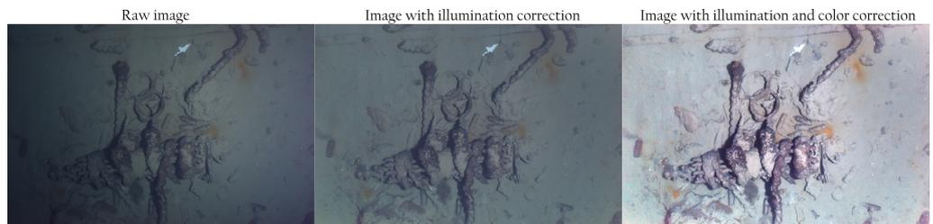
**Figure 5.** Example of image correction techniques implemented in *Matisse*. The raw image (**left**) is corrected for uneven illumination only (**center**) or for both illumination and color correction (**right**).
