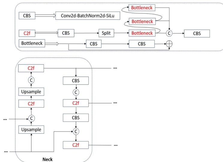
**Figure 8.** Diagram of the neck structure after improving the key modules.
