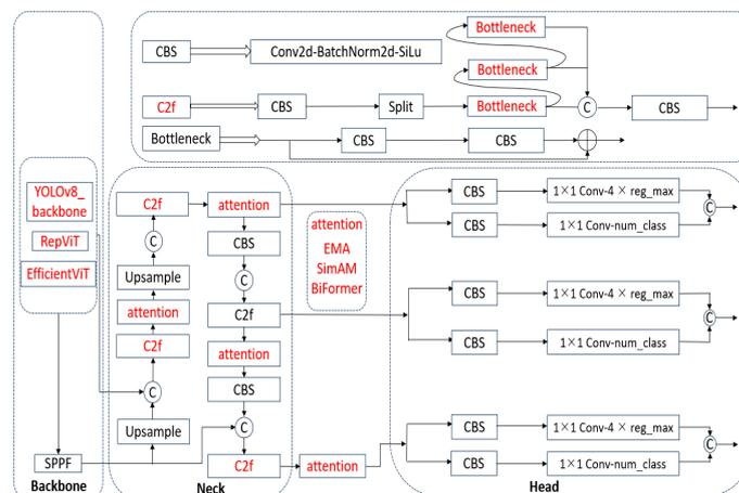
Figure 12. YOLOv8 weed detection model structure with different improvement methods.
