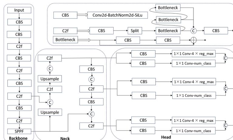
Figure 4. Overall structure of YOLOv8.
