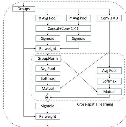
Figure 10. EMA module structure.
