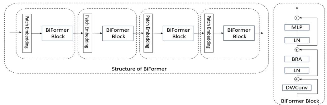
Figure 11. BiFormer module structure.
