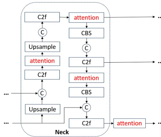
Figure 9. YOLOv8 neck structure after improving C2f module.
