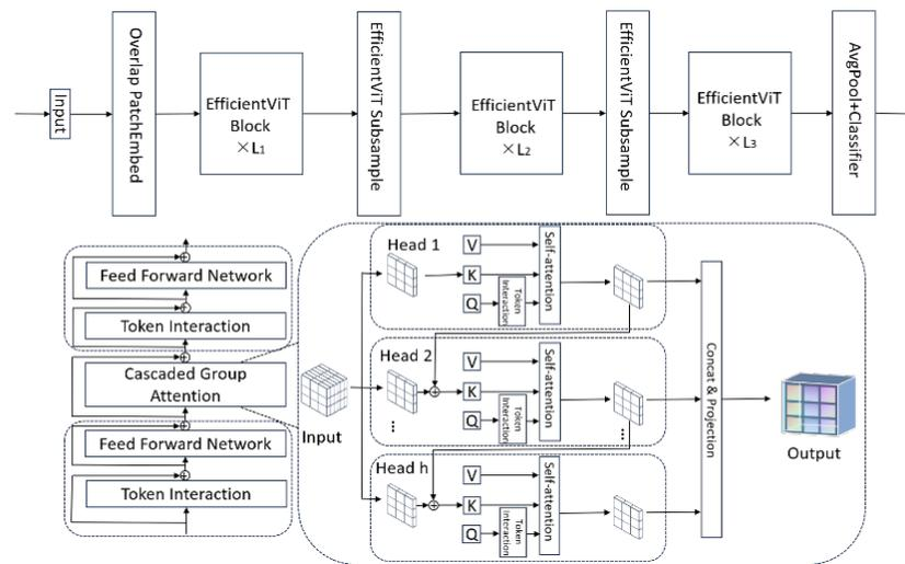
**Figure 6.** EfficientViT network structure.
