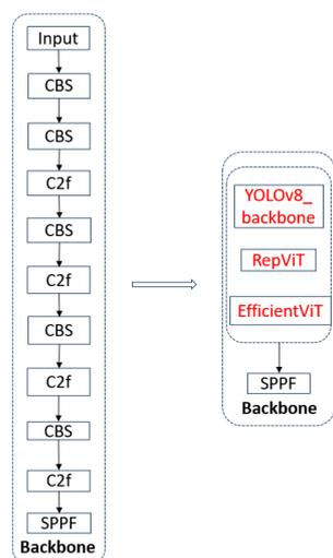
**Figure 5.** The overall structure of the YOLOv8 backbone network after improvement.
