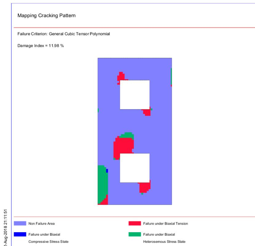
Figure 29. Mapping cracking pattern based on general cubic tensor polynomial failure criterion.
