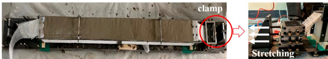
Figure 3. Textile-reinforced mortar (TRM)-strengthening device with textile stretching.
