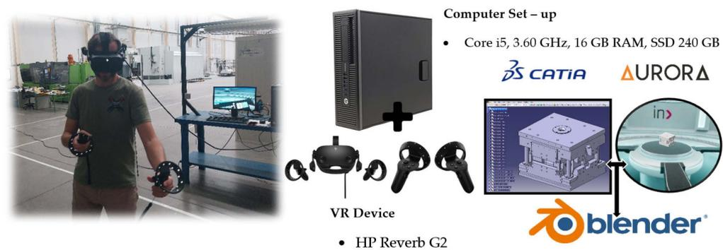
**Figure 3.** CAD—VR devices and environment.
