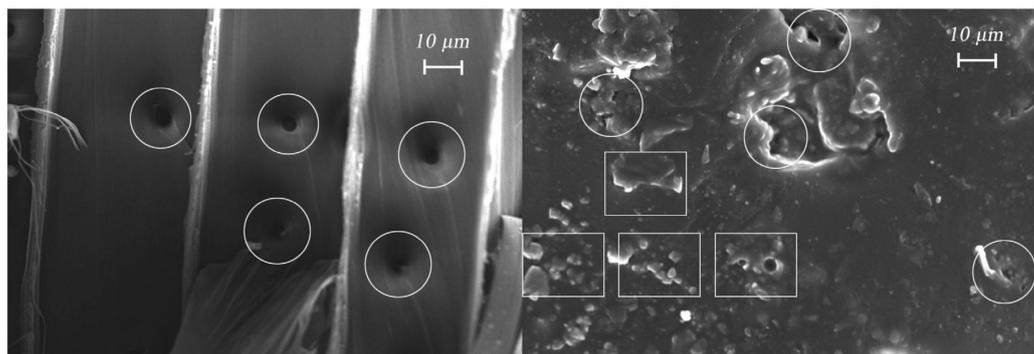
**Figure 2.** SEM micrographs of untreated wood (**left**) and of the wood after treatment with tung oil (**right**) [49]. From *Industrial Crops and Products*, 140, Z. He, J. Qian, L. Qu, N. Yan, S. Yi, *Effects of Tung oil treatment on wood hygroscopicity, dimensional stability and thermostability*, 111647, Copyright (2019), with permission from Elsevier.
