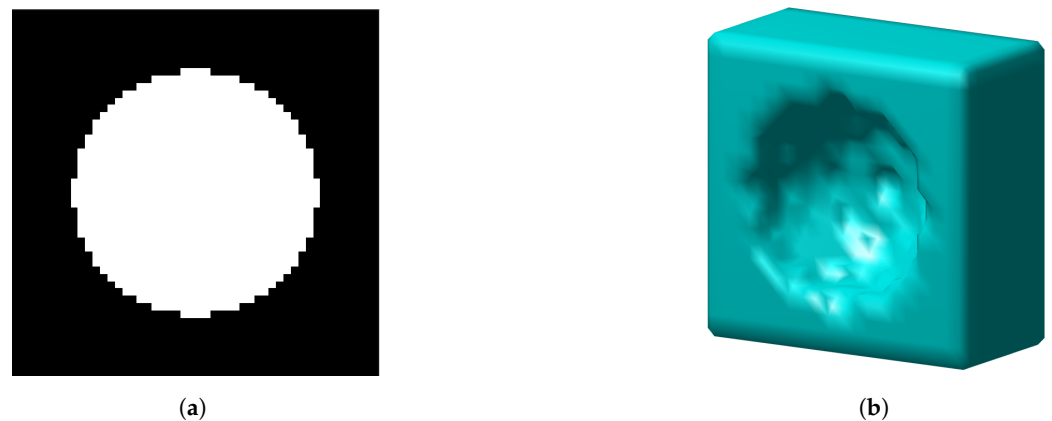
Figure 1. Initial geometries of the periodic unit cell. (a) Initial geometry of 2D periodic unit cell. (b) Initial geometry of 3D periodic unit cell.
