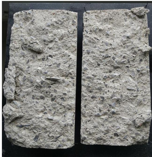
**Figure 15.** Breaking surface of a cylindrical specimen after a tensile splitting strength test.
