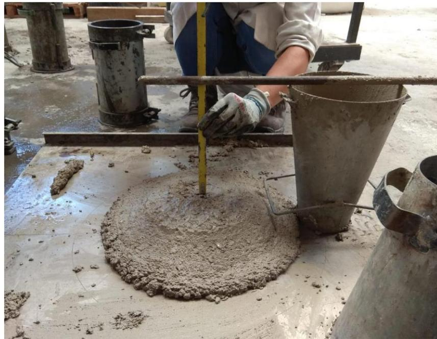
**Figure 6.** Measuring the height of the Abrams cone test.
