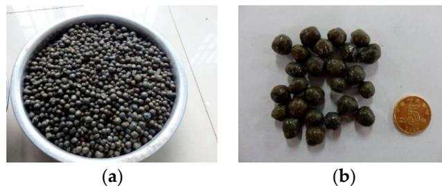
**Figure 11.** LWA appearance in the different binders: (a) LWA treated by the pre-wetting method; (b) LWA treated by a sodium silicate solution.
