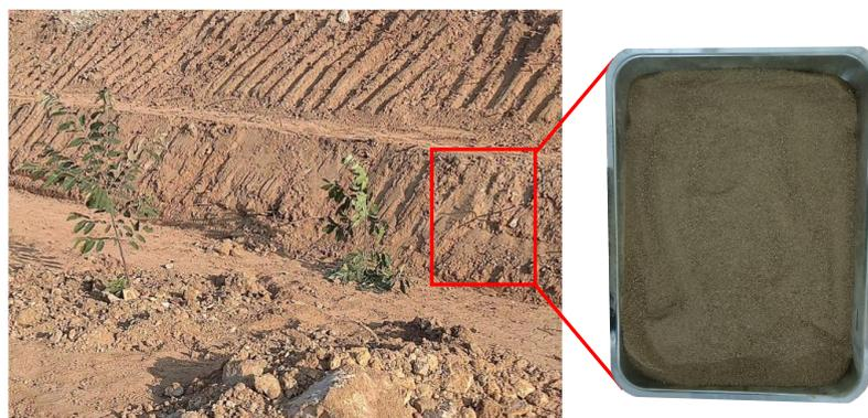
**Figure 1.** Untreated soil specimens and the expansion site of the Rongwu Expressway's Weihai–Yantai section.
