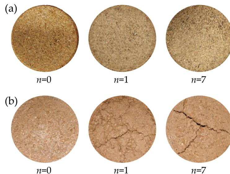
**Figure 6.** Pictures of soil samples with varying numbers of cycles ( $n$ ). (a) sandy clay soil; (b) clay soil that is powdery.
