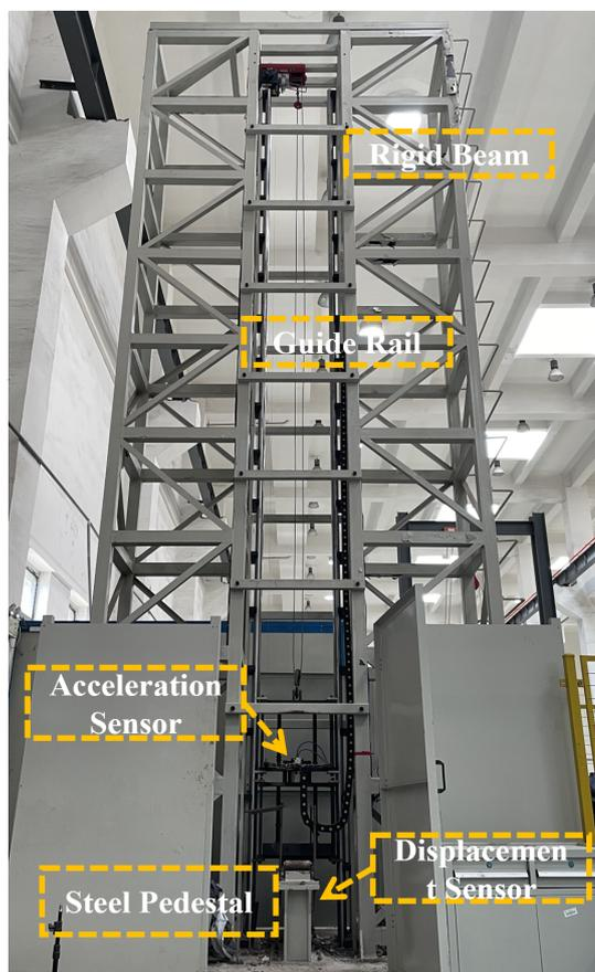
(a) Drop weight impact test loading device
