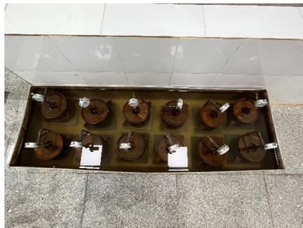
**Figure 4.** The CBR specimens.
