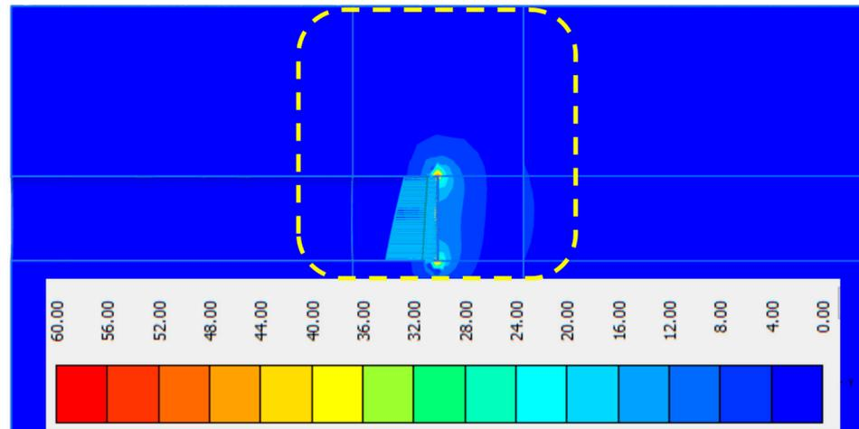
**Figure 5.** Distribution nephogram of hydraulic gradient at the position of tunnel face under limit state [ $\chi = 1.0 D$ ].
