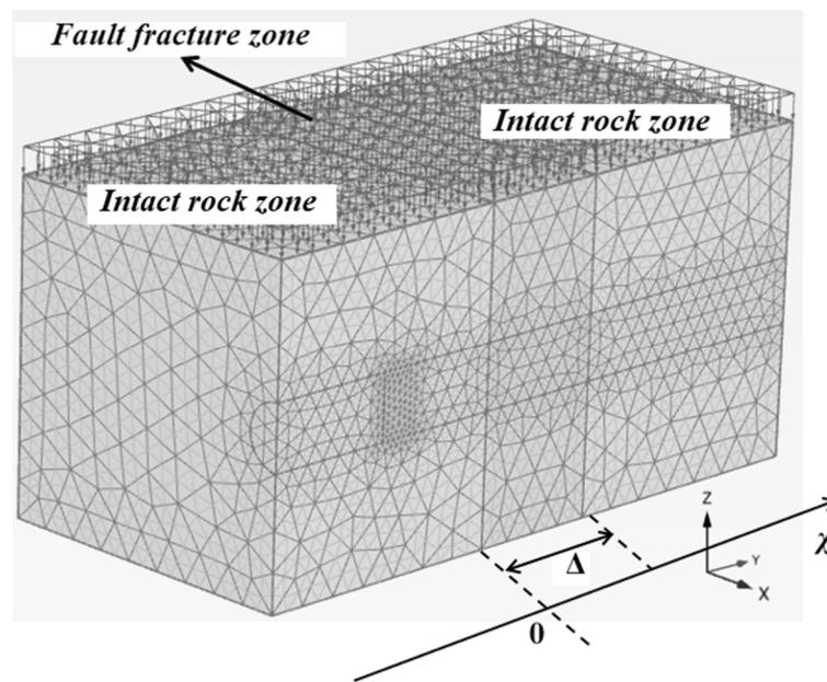
**Figure 2.** Finite element numerical simulation model.
