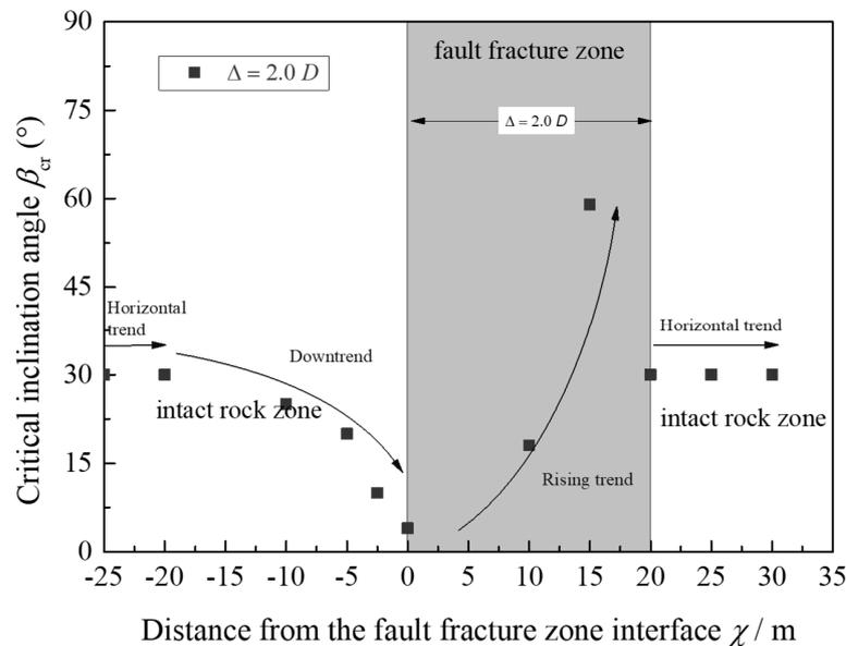
**Figure 12.** Critical inclination angle  $\beta_{cr}$  with different locations of the tunnel face in the limit state.
