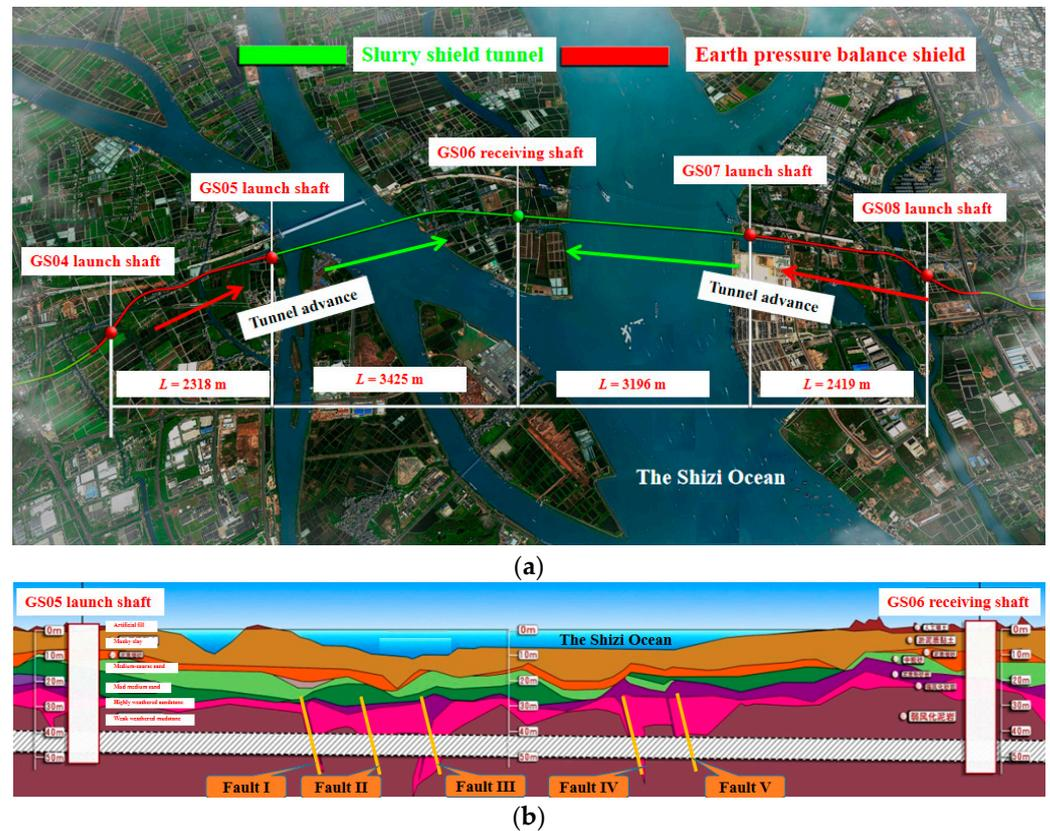
**Figure 1.** A tunnel engineering project with several zone of fault fractures with high hydraulic pressure. (a) Plan view of project site; (b) Geological profile.
