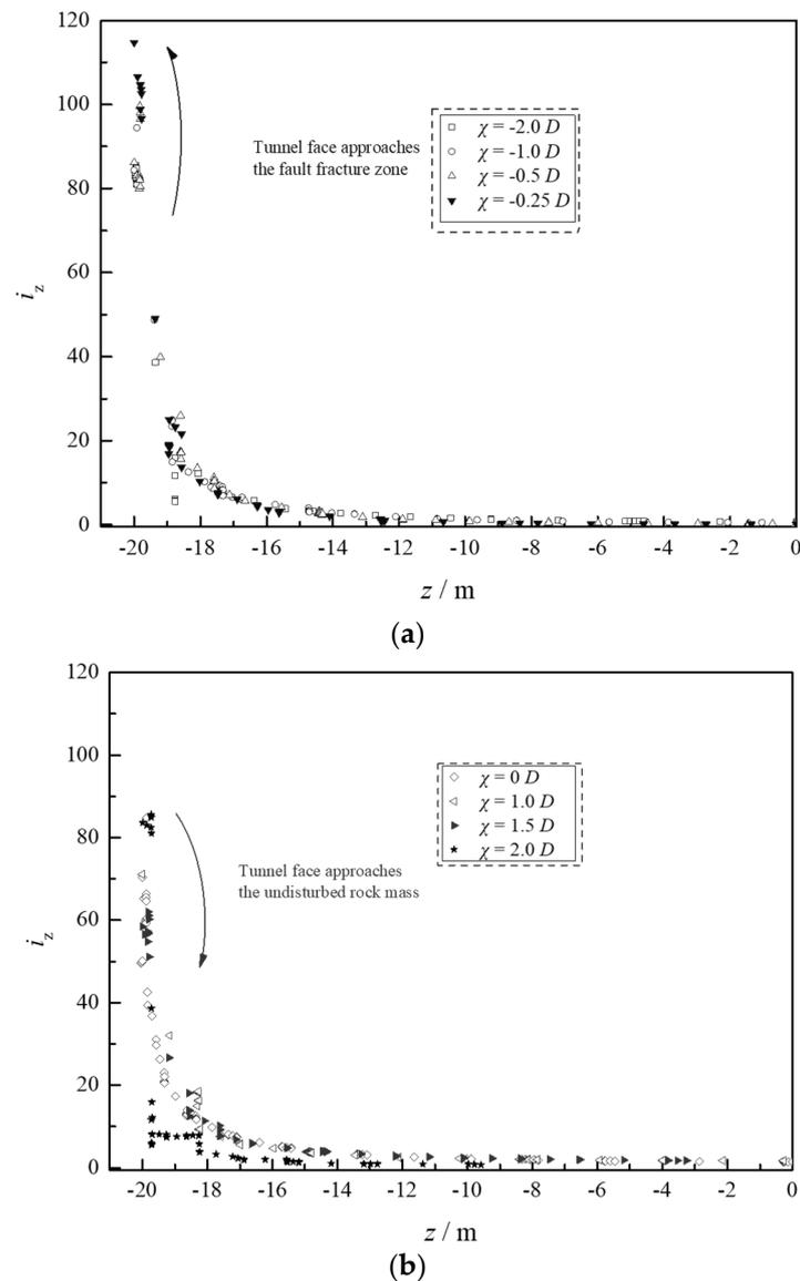
**Figure 7.** Hydraulic gradients on vertical measuring lines at different distances: (a) when the tunnel face is advanced towards the fault fracture zone; (b) when the tunnel face is advanced towards the area of undisturbed rock mass.
