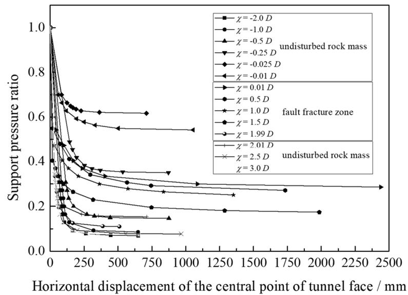
Figure 8. Relation between horizontal displacement and support pressure ratio ( $L = 2.0 D$ ).
