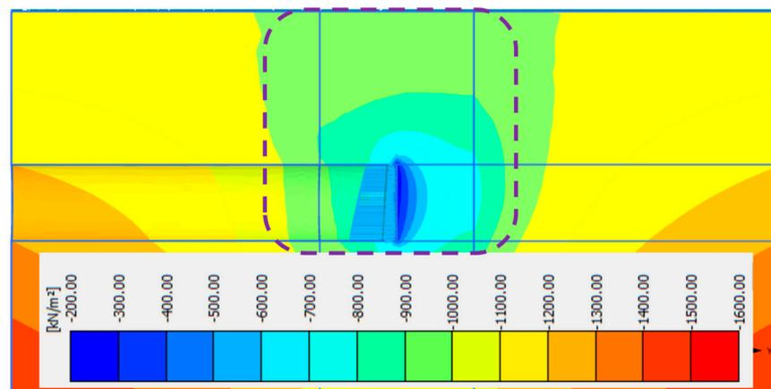
**Figure 4.** Distribution nephogram of pore water pressure at the position of tunnel face under limit state [ $\chi = 1.0 D$ ].
