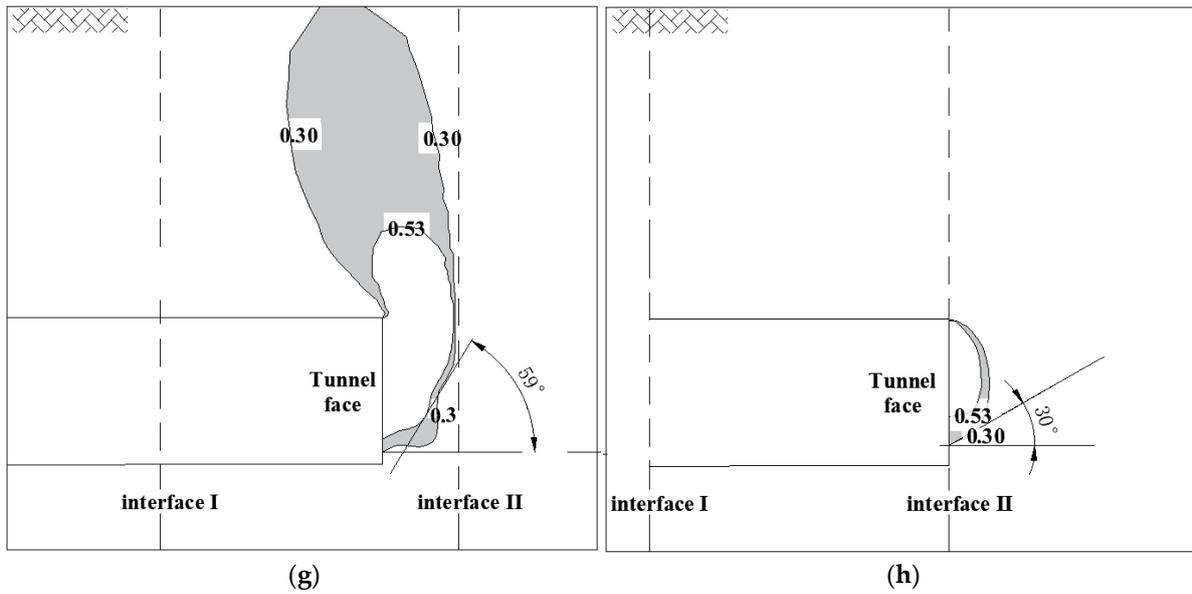
**Figure 11.** Failure zone boundary at different positions of tunnel face in limit state. (a)  $\chi = -2.0 D$ ; (b)  $\chi = -1.0 D$ ; (c)  $\chi = -0.5 D$ ; (d)  $\chi = -0.25 D$ ; (e)  $\chi = 0 D$ ; (f)  $\chi = 1.0 D$ ; (g)  $\chi = 1.5 D$ ; (h)  $\chi = 2.0 D$ .
