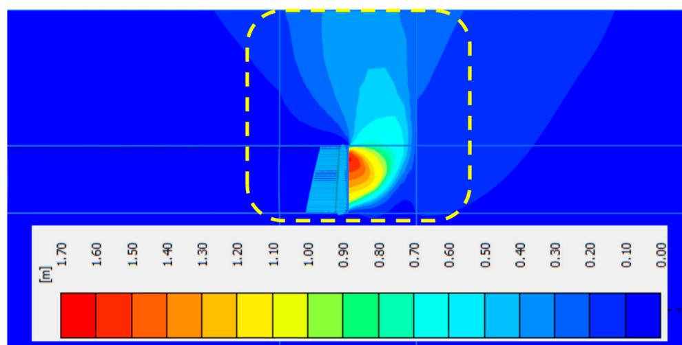
**Figure 10.** Nephogram of stratum displacement distribution at different positions of tunnel face under limit state [ $\chi = 1.0 D$ ].
