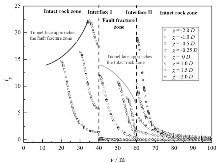
**Figure 6.** Hydraulic gradients on measurement lines at different distances from launching planes.
