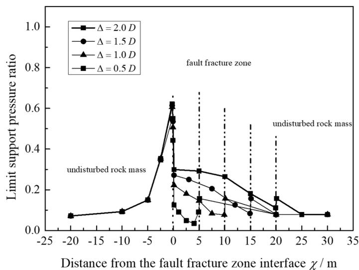
Figure 9. Influence of the width of zone of fault fracture on the variation of limiting support force.
