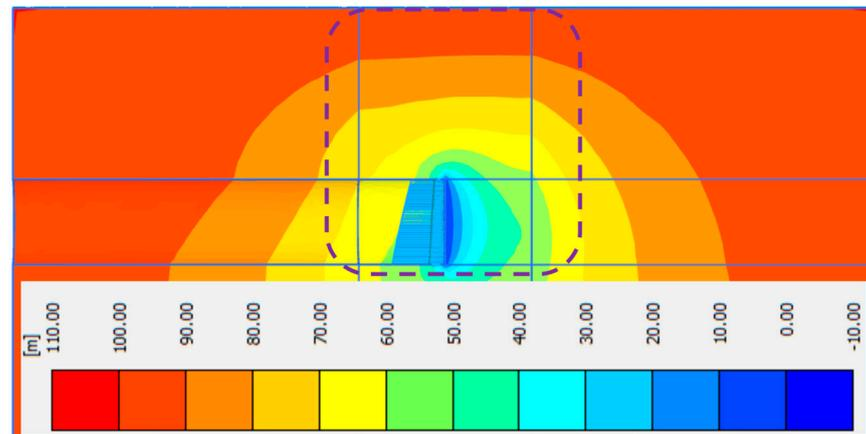
**Figure 3.** Nephogram of water head distribution at the position of tunnel face under limit state [ $\chi = 1.0 D$ ].
