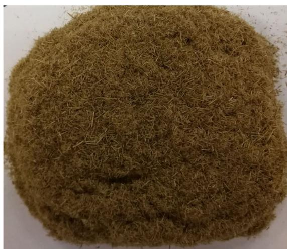
**Figure 1.** Photograph of original bagasse fibers.
