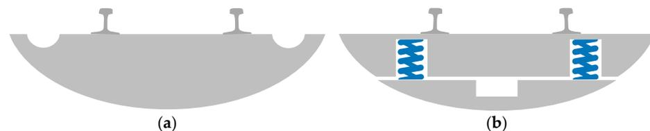
**Figure 4.** Cross-sections of two track beds: (a) GIT and (b) SSFT.
