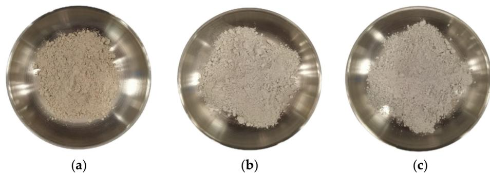
**Figure 1.** Three different particle sizes of tuff powder (a) CT, (b) MT, and (c) FT.
