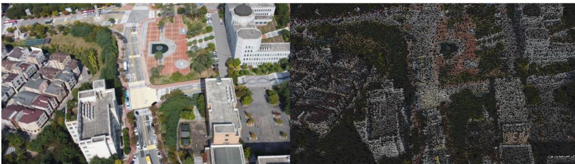
Figure 23. GAN training dataset: drone-captured photo (left); photo after adding point cloud noise (right).
