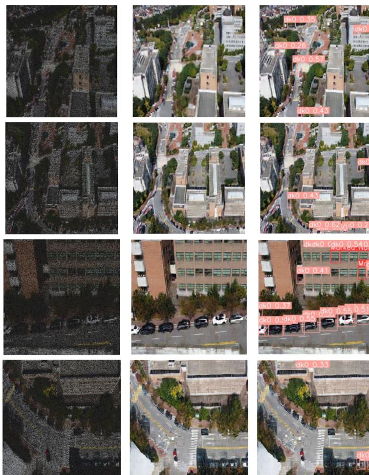
**Figure 24.** Before photorealistic rendering (left); after photorealistic rendering (middle); object detection from photorealistic rendered PCM model (right).
