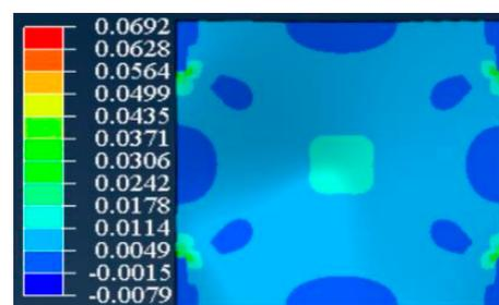
**Figure 13.** Stress field diagram of FEA of CFRP laminates under mid-point load.
