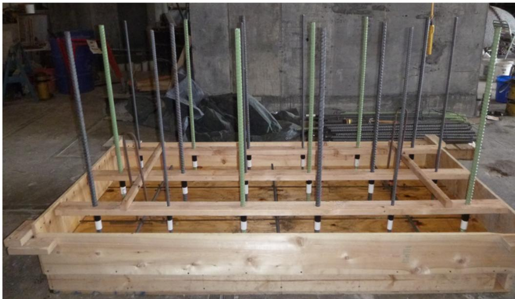
**Figure 9.** Pull-out slab specimen dimensions and bar arrangement (PHASE III) (1 in. = 25.4 mm).
