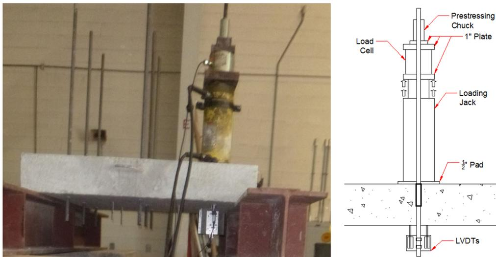
**Figure 8.** Pull-out wall specimen test setup (PHASE II).
