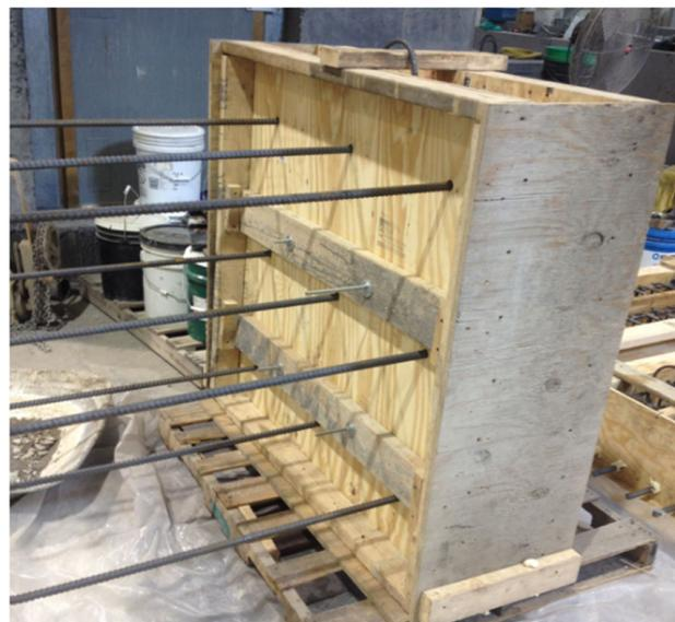
**Figure 6.** Pull-out wall specimen formwork (PHASE II).
