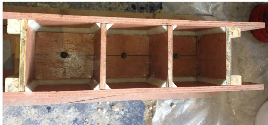
Figure 4. Pull-out cube specimens' formwork (PHASE I).
