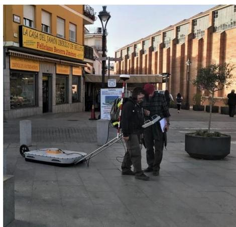
**Figure 7.** The use of GPR at Margarita Xirgú Square in Mérida to detect possible archaeological remains in the drafting phase of the project for the remodelling and adaptation of the square as a tourist reception area.
