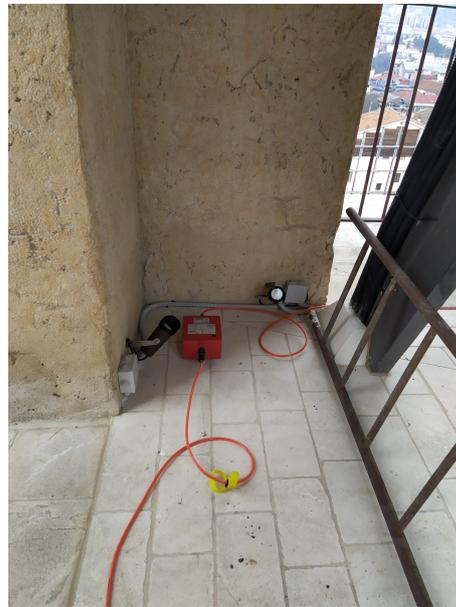
Figure 19. Accelerometer placed on the top of the bell tower, at the height of 22.03 m.
