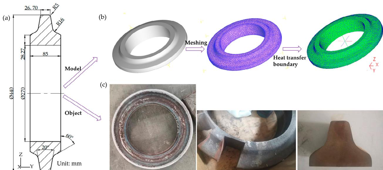
**Figure 3.** (a) Dimensional diagram of shield machine cutter ring; (b) simulation model, finite element meshing and the scheme of heat transfer; and (c) the object of the shield machine cutter ring.
