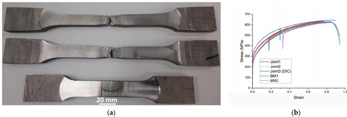
**Figure 5.** Tensile curves of 304L SS SAW joints and BM. (a) Tensile specimens before and after the test and (b) tensile curves.
