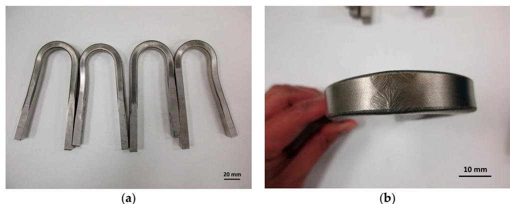
**Figure 6.** Transverse side bend-tested AISI 304/304L SS welded joint specimens: (a) bend-tested specimens and (b) deformed welded joint.
