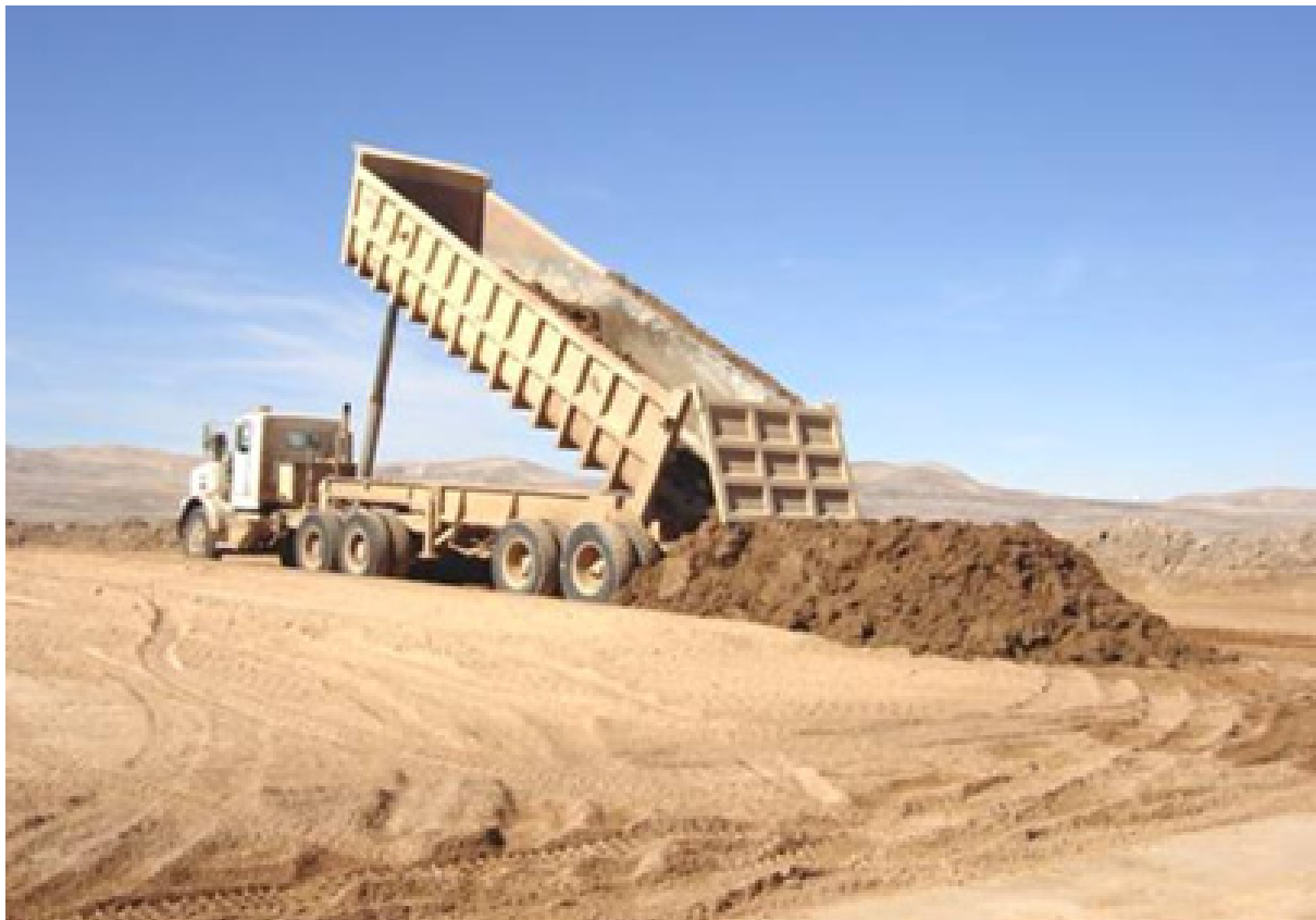
Figure 32. El Peñon Filtered Tailings Storage Facility—Haul Truck with Tails Disposal [62,63].
