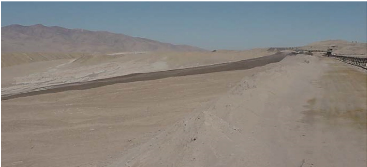
Figure 49. Mantos Blancos Disposal of Filtered Coarse Tailings with Mobile Stacker Conveyor and Tripper [18,67,68].
