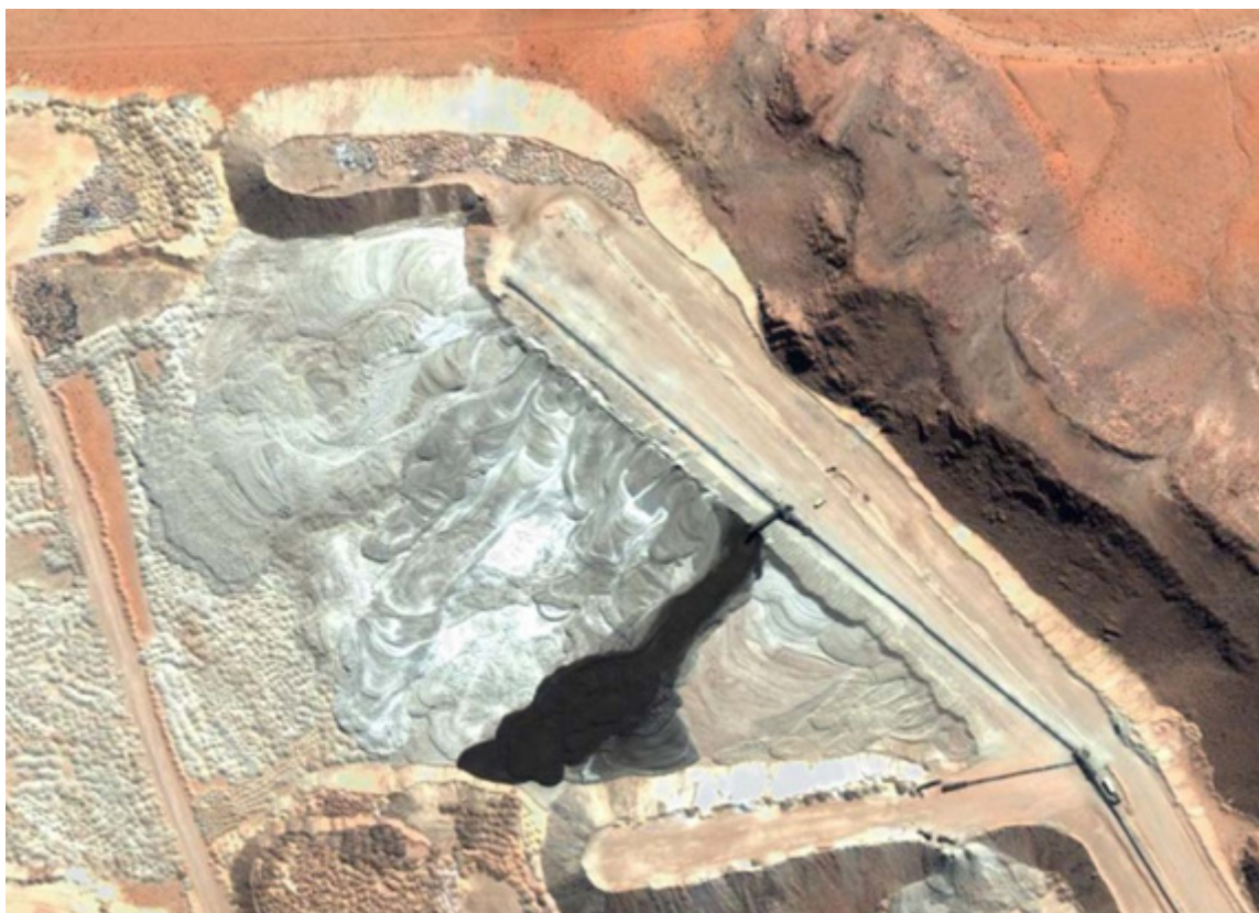
Figure 50. Mantos Blancos Aerial View of Disposal of Filtered Coarse Tailings [18,67,68].
