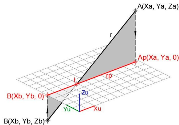
**Figure 20.** Checking whether line  $r$  and meshed plane are parallel.
