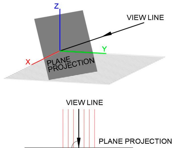
Figure 5. View line and perpendicular projection plane.
