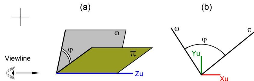
**Figure 33.** Angle  $\varphi$  between two planes  $\pi$  and  $\omega$ : (a) UCS Z axis matches to the intersection line of both planes; (b) angle  $\varphi$  measurement is shown in top view.
