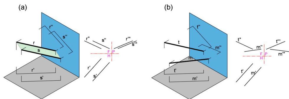
**Figure 18.** (a) Lines  $r$  and  $s$  are parallel. (b) Lines  $t$  and  $m$  are not parallel.
