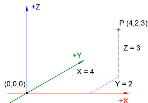
**Figure 4.** Point P (4, 2, 3) location in the Cartesian coordinate system.
