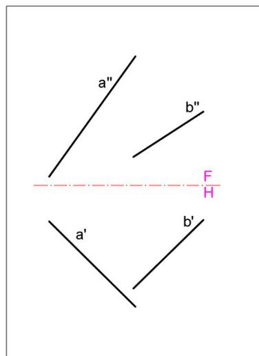
**Figure 24.** Problem statement: the top and front views of skew lines  $a$  and  $b$ .
