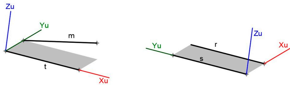
**Figure 19.** Using the UCS for checking parallelism between lines. Lines  $m$  and  $t$  are not parallel, while lines  $r$  and  $s$  are.
