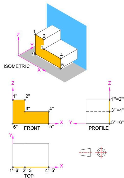
**Figure 1.** Views obtained from orthographic first-angle projection.
