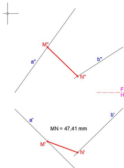
Figure 30. Top and front views and true length dimension of segment  $MN$ .
