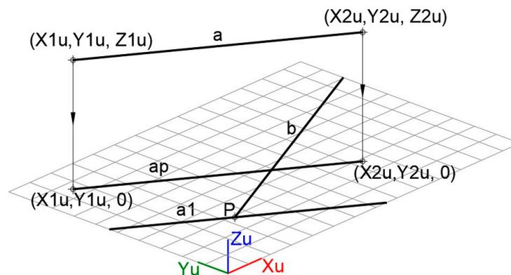
**Figure 27.** Projection *ap* of line *a* onto the plane defined by *a1* and *b*.
