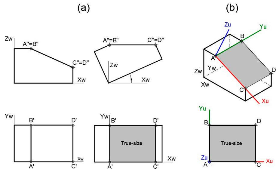
**Figure 17.** True size of the plane ABCD by (a) rotating the body without modifying the coordinate system; and (b) considering an UCS.
