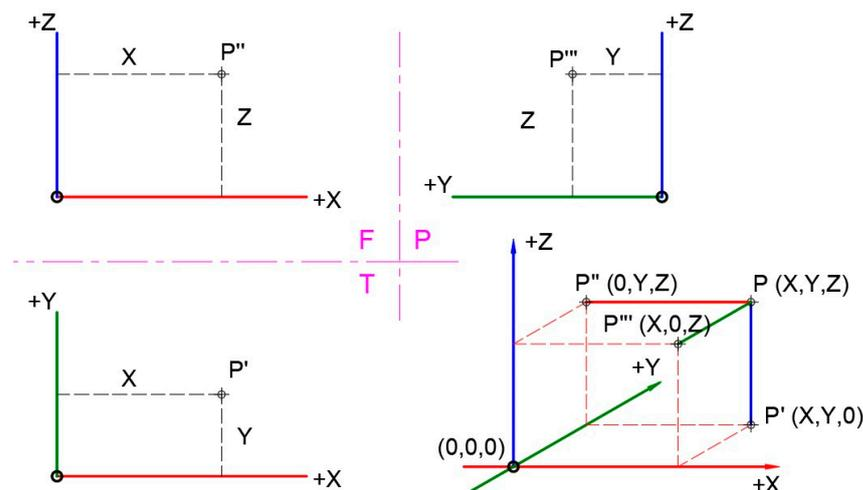
**Figure 12.** Cartesian coordinates in a multi-view drawing.
