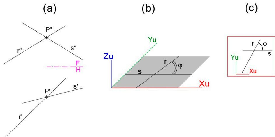
**Figure 31.** Angle between two coplanar lines  $r$  and  $s$ : (a) top and front view of  $r$  and  $s$ ; (b) matching UCS to the plane defined by  $r$  and  $s$ ; and (c) angle  $\varphi$  measurement in the top view of the UCS.
