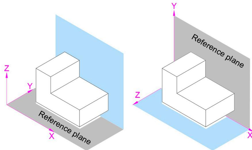
**Figure 3.** Examples for reference plane positions.
