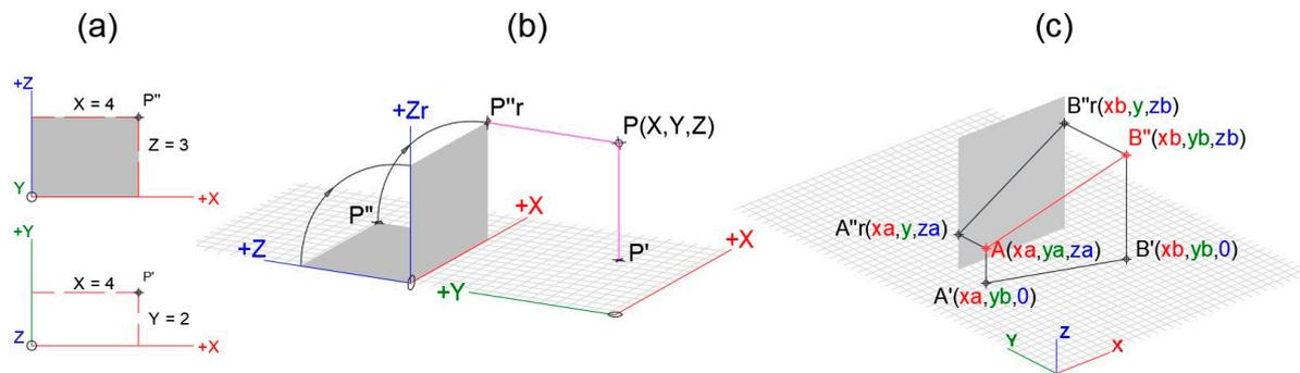
**Figure 11.** (a) Orthographic projections of a point; front view coordinates X, Z and top view coordinates X, Y. (b) Front view rotated  $90^\circ$  with respect to the X axis. (c) Application to an oblique line defined by points A and B.
