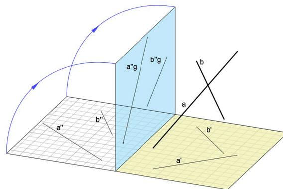
**Figure 25.** Line *a* and *b* restitution for obtaining their 3D positions.
