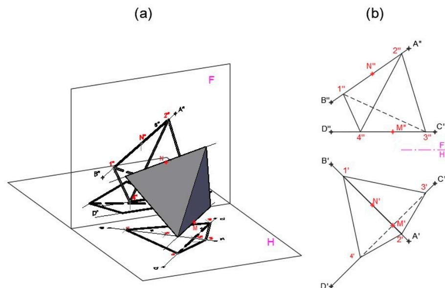
**Figure 34.** Regular polyhedra problem solved with CADOP: (a) tetrahedron obtained in 3D, knowing that two of its opposite edges are located on two perpendicular skew lines; (b) top and front views of the polyhedron solution.
