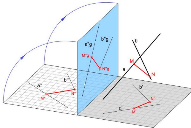
Figure 29. Three-dimensional position of perpendicular line and shortest distance segment  $MN$  between skew lines  $a$  and  $b$ .
