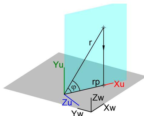
**Figure 32.** Angle between line and plane: angle  $\varphi$  measurement in the top view of the UCS defined by line  $r$  and its projection  $rp$  onto a plane.
