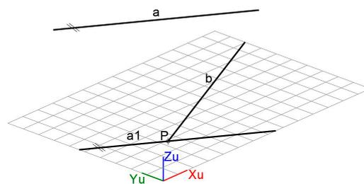
**Figure 26.** Plane through line *b* parallel to line *a*.
