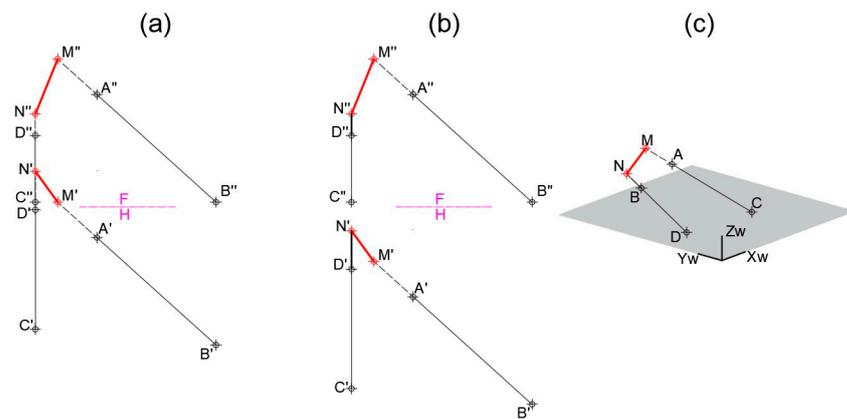
**Figure 23.** Solution obtained using CADOP for the perpendicular line and shortest distance between two skew lines  $r$  and  $s$ . (a) Hiding the layers in which intermediate steps are drawn. (b) Arranging the views for avoiding projections overlapping. (c) Three-dimensional view.
