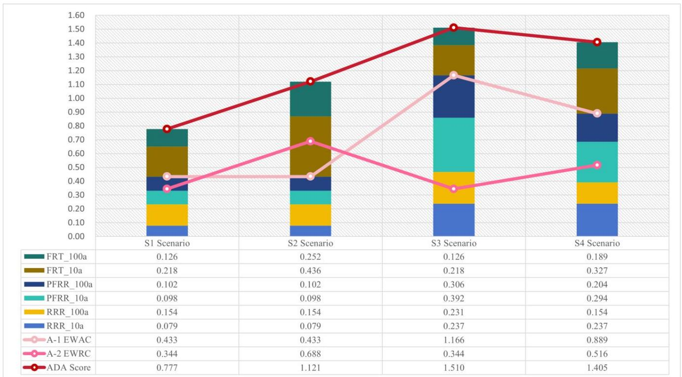
**Figure 7.** Environmental resilience index of ADA indicators. Note: RRR\_10a = runoff reduction rate 10a; RRR\_100a = runoff reduction rate 100a; PFRR\_10a = peak flow reduction rate 10a; PFRR\_100a = peak flow reduction rate 100a; FRT\_10a = flood recovery time 10a; FRT\_100a = flood recovery time 100a; EWAC = extreme weather adaptation capability; EWRC = extreme weather recovery capability; and ADA = acute disturbance adaptation.
