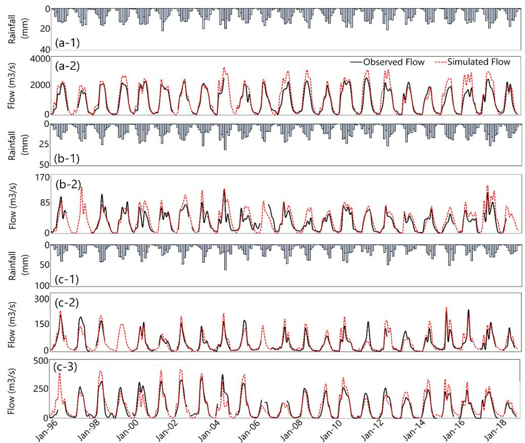
Figure 3. Observed versus Simulated Flow at Sheola (a-2) in the Barak sub-basin, at Kamalganj (b-2) in the Tripura sub-basin, and at Islampur (c-2) and Muslimpur (c-3) in the Meghalaya sub-basin. Here, the upper panels (a-1,b-1,c-1) represent the basin averaged monthly precipitation.
