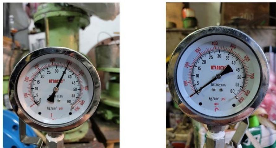
**Figure 9.** Water pressure gauge readings at both sides of jacket during pressure testing.
