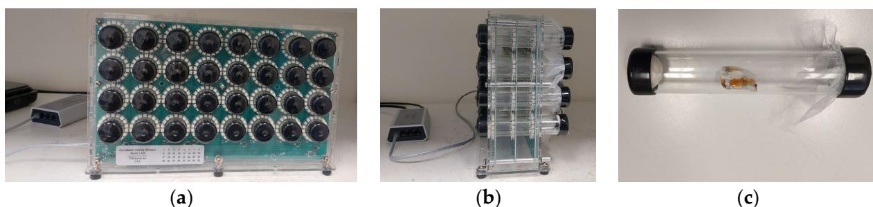
**Figure 3.** Front (a) and side view (b) of the Trikinetics (LAM25system) set in laboratory. The tube setup: vinyl plastic stoppers (black color) were placed on one end (a,b) and cups with organdy cloth placed on the other end for the ventilation of the tubes (c) (photos taken by E. Balampelou).
