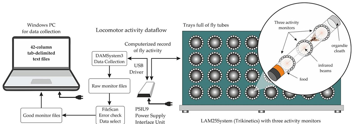
**Figure 4.** Locomotor activity dataflow using LAM25 System (Trikinetics).
