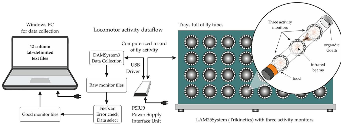
**Figure 4.** Locomotor activity dataflow using LAM25 System (Trikinetics).
