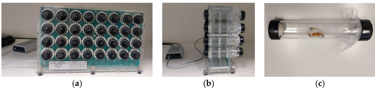
**Figure 3.** Front (a) and side view (b) of the Trikinetics (LAM25) system set in laboratory. The tube setup: vinyl plastic stoppers (black color) were placed on one end (a,b) and cups with organo cloth placed on the other end for the ventilation of the tubes (c) (photos taken by E. Balampekou).
