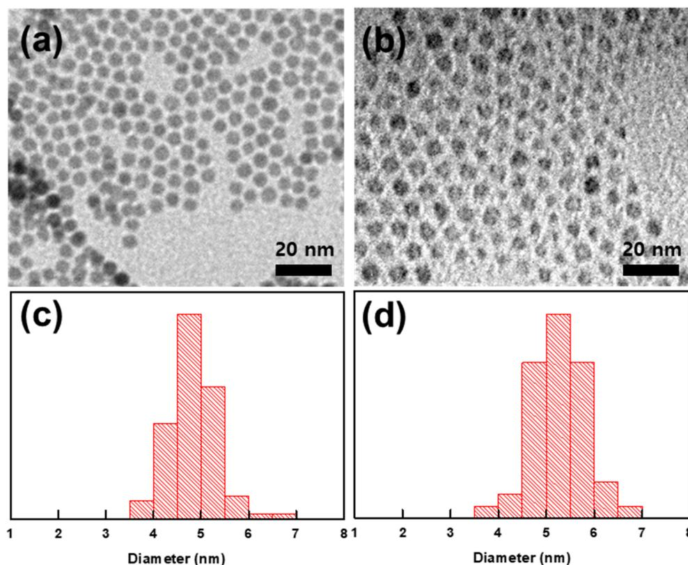
**Figure 2.** (a,b) TEM image and (c,d) size distribution histogram of (a,c) Au NPs and (b,d) Fe<sub>3</sub>O<sub>4</sub> NPs.
