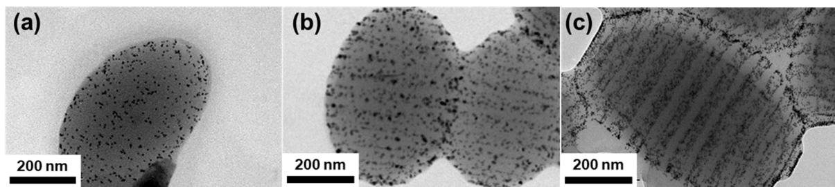
**Figure 4.** TEM images showing the distribution of Au NPs in PS-*b*-PB/Au ellipsoids as a function of the volume fraction of NP relative to BCP ( $\phi$ ). (a) 1.4 vol%, (b) 3.5 vol%, and (c) 7.0 vol%. Particles were observed without staining.  $A_{\text{emul/air}} = 26.4 \text{ cm}^2$ .
