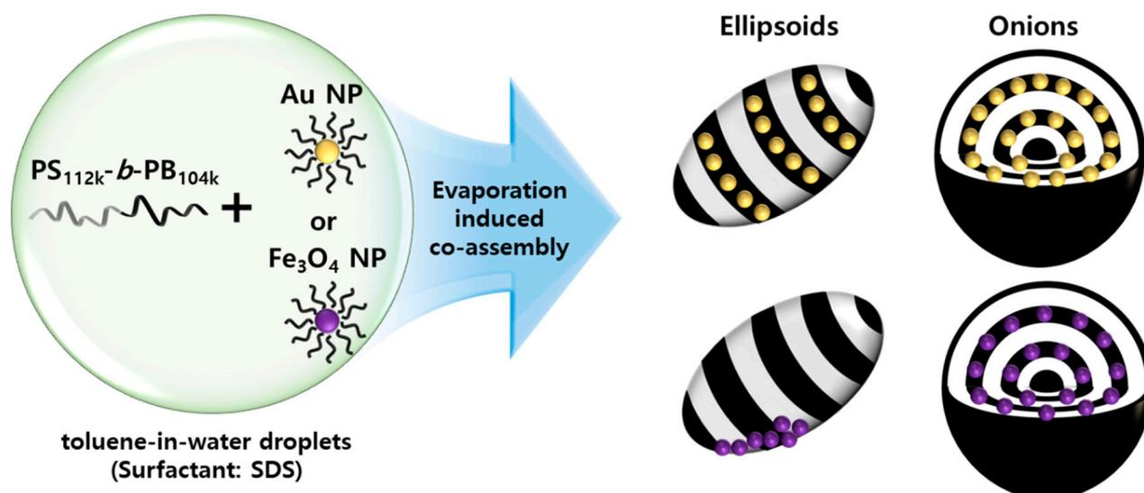
**Figure 1.** Illustration showing co-assembly of inorganic nanoparticles (Au NP and  $\text{Fe}_3\text{O}_4$  NP) with PS-*b*-PB BCPs by controlled solvent evaporation from toluene-in-water emulsion.
