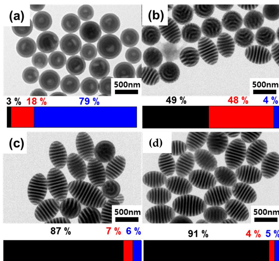
**Figure 5.** TEM images of hybrid PS-*b*-PB/Au particles as a function of  $\phi$ . (a) Pristine PS-*b*-PB particles, (b)  $\phi = 1.4$  vol%, (c)  $\phi = 3.5$  vol%, and (d)  $\phi = 7.0$  vol%. Each color of the bar chart shows the percentage of each morphology. Black: ellipsoids, red: intermediates, blue: onions. PB domains were stained with OsO<sub>4</sub>.  $A_{\text{emul/air}} = 0.1$  cm<sup>2</sup>.
