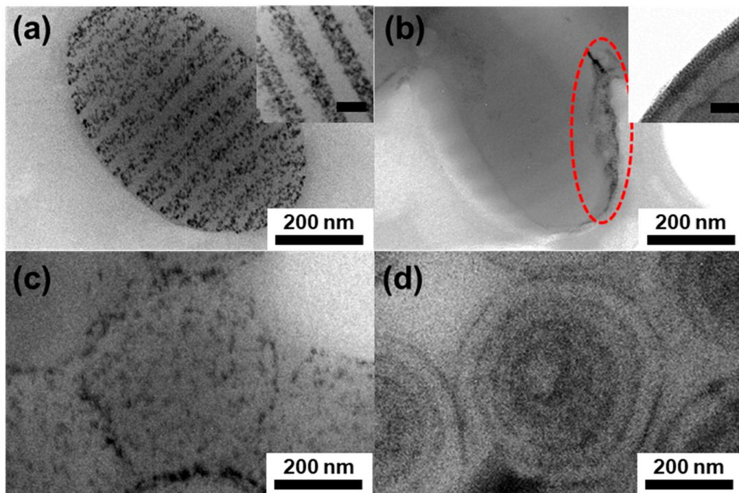
**Figure 3.** TEM images showing hybrid PS-*b*-PB particles. Striped ellipsoids (a,b) and onion-like particles (c,d) containing (a,c) Au NP or (b,d) magnetic NPs. Fe<sub>3</sub>O<sub>4</sub> NPs were segregated at the edge of the ellipsoidal particles as indicated by red dashed circles in Figure 3b. The loading amount of NPs was fixed to 7.0 vol% for both Au and Fe<sub>3</sub>O<sub>4</sub>. Particles were observed without staining. Scale bars in inset figures are 50 nm.
