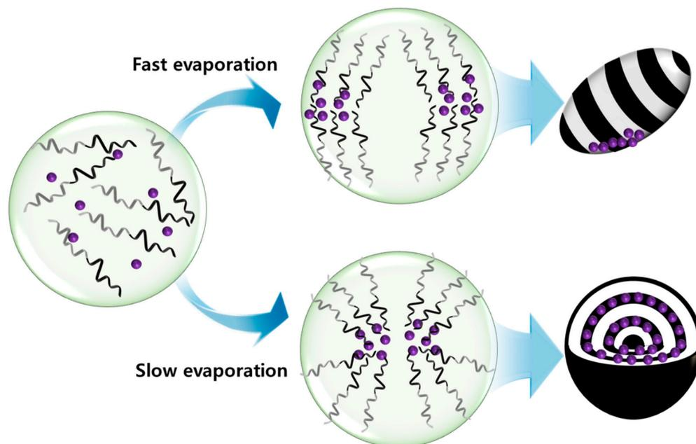
**Figure 7.** Schematic illustration showing the formation mechanism of PS-*b*-PB/Fe<sub>3</sub>O<sub>4</sub> ellipsoids and onion-like particles.
