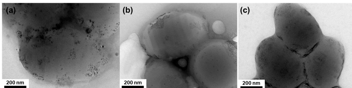
**Figure 6.** TEM images showing the distribution of  $\text{Fe}_3\text{O}_4$  NPs in PS-*b*-PB striped ellipsoids as a function of  $\varphi$ . (a) 1.4 vol%, (b) 3.5 vol%, and (c) 7.0 vol%. Particles were observed without staining.
