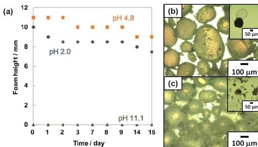
**Figure 2.** (a) Temporal change of foam height observed for the foams prepared at pH 2 (●), pH 4.8 (■), pH 11.1 (▲). (b,c) Optical micrographs of bubbles stabilized with ACMPA-PS particles prepared at (b) pH 2.0 and (c) 4.8. Insets of (b,c) show the bubbles between glass substrates after the application of pressure. An inset of (b,c) shows the bubbles after the application of pressure between glass substrates.
