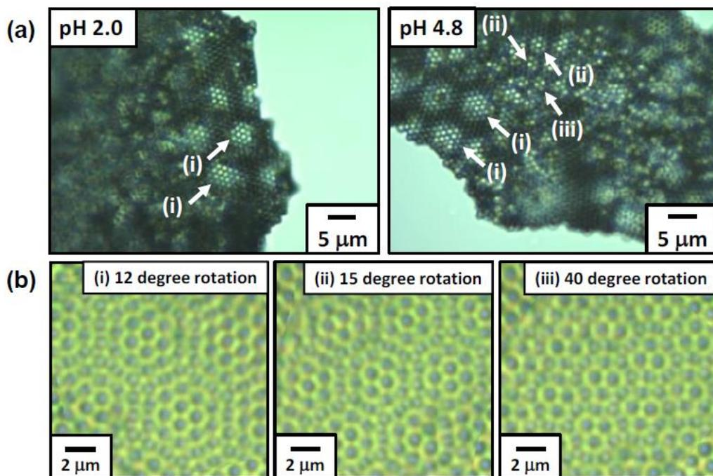
**Figure 6.** (a) Moiré patterns produced by ACMPA-PS particle bilayers as observed by optical microscopy. (b) Simulation images obtained by superimposing a semi-transparent (40% transmission) optical micrograph image of a hexagonally ordered particle array onto the identical non-transparent image after rotation of the semi-transparent image through angles of 15, 40 and 50° relative to the non-transparent image.
