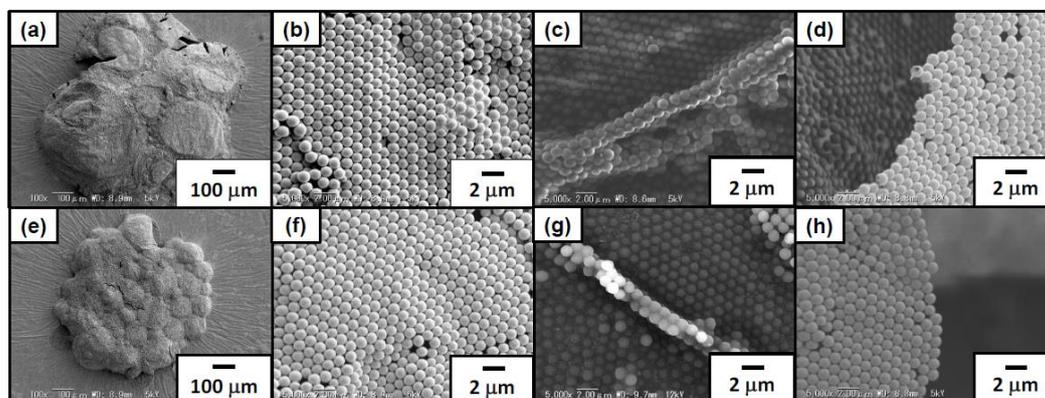
**Figure 3.** Scanning electron microscope (SEM) images of dried foams stabilized with ACMPS-PS particles prepared at (a–d) pH 2.0 and (e–h) pH 4.8. (b,f) are magnified images of (a,e). (c,d,g,h) are cross-section SEM images of the foams after deliberate rupture using a razor blade.
