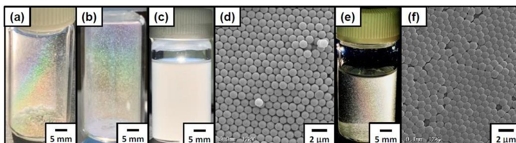
**Figure 7.** Digital photographs of ACMPA-PS particle-stabilized foam fragments prepared at pH 2.0 viewed under (a,c,e) white light and (b) sunlight. The fragments were dispersed in ethanol (c) before and (e) after annealing with toluene vapor for 15 min. SEM images of foam fragments (d) before and (f) after the annealing with toluene vapor.
