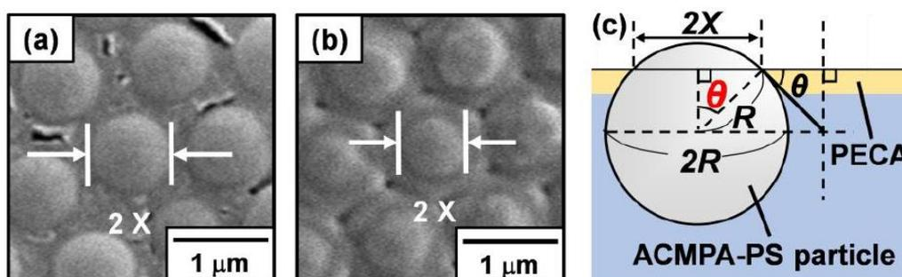
**Figure 5.** SEM images of ACMPA-PS particles prepared at (a) pH 2.0 and (b) 4.8 trapped with poly(ethyl 2-cyanoacrylate) (PECA) films recorded from the air-exposed side of the films. (c) Determination of the contact angle (through water) of the ACMPA-PS particle at the air–water interface using SEM images.
