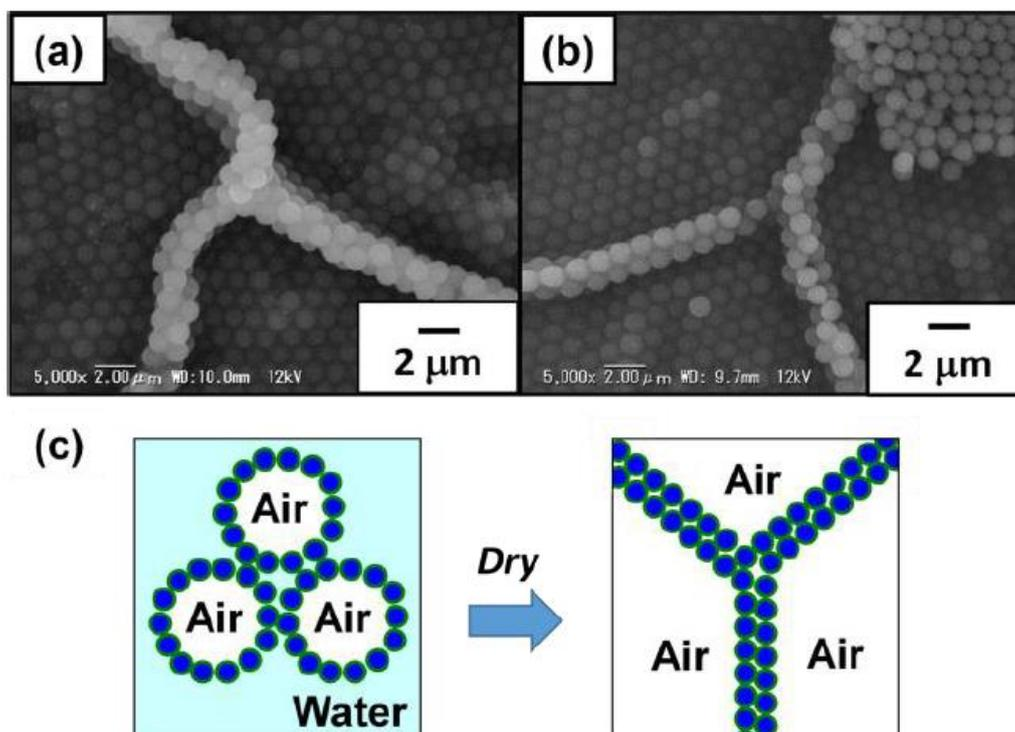
**Figure 4.** Cross-sectional SEM images of dried foams stabilized with ACMPA-PS particles prepared at (a) pH 2.0 and (b) pH 4.8 after rupturing using a razor blade. (c) Scheme illustrating formation of bilayers of ACMPA-PS particles array via drying.
