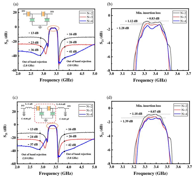
**Figure 7.** Measured transmission responses ( $S_{21}$ ) of the fabricated FBAR filters. (a) The  $S_{21}$  responses of the filters with different orders. (b) The enlarged view of the passband in (a). (c) The  $S_{21}$  responses of the filters in (a) with the external circuit compensation. (d) The enlarged view of the passband in (c).
