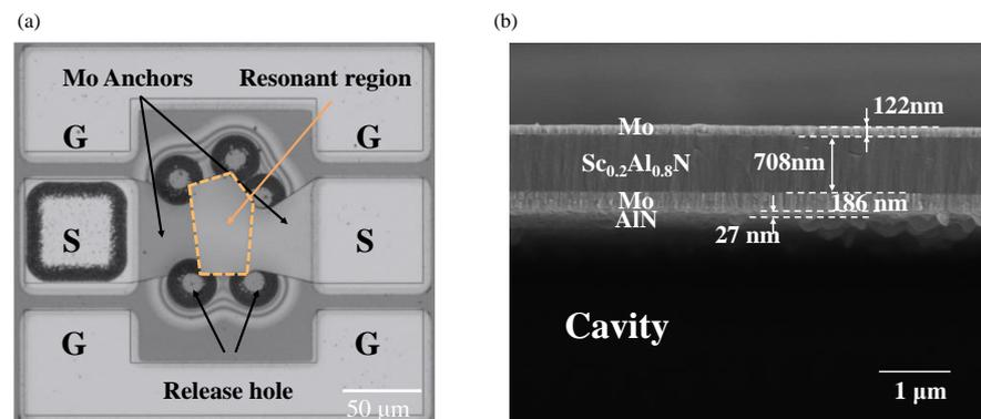
**Figure 4.** Characteristics of fabricated FBARs. (a) SEM image of top view of the fabricated FBAR resonator. (b) SEM image of the cross-sectional view of the fabricated FBAR resonator.
