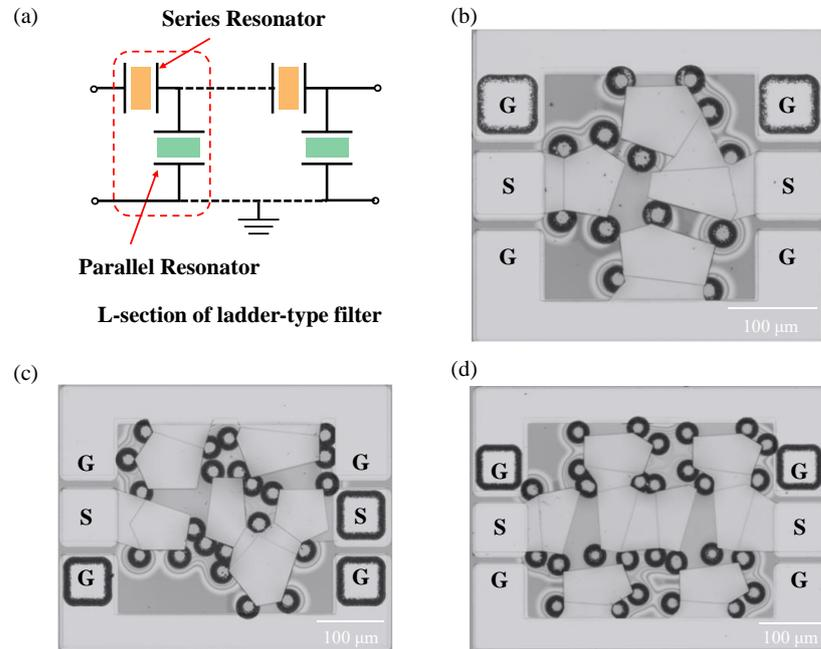
**Figure 6.** FBAR filters with different topological structures. (a) Schematic circuit designs of the FBAR filter. (b–d) Second-, third- and fourth-order ladder-type FBAR filters, respectively.
