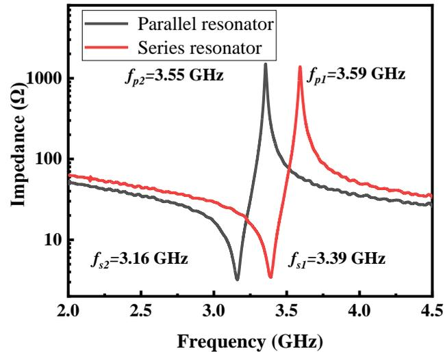
Figure 5. Measured impedance response of series and parallel resonators.
