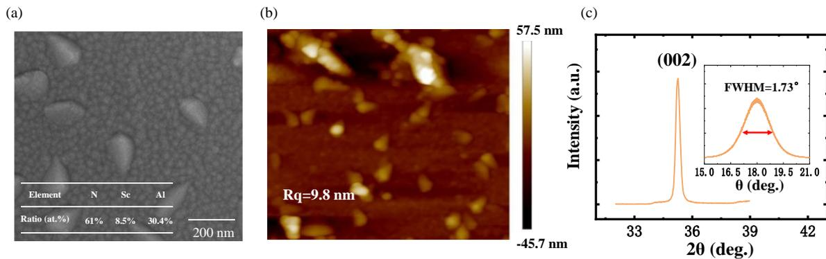
**Figure 3.** Characterization of the prepared  $\text{Sc}_{0.2}\text{Al}_{0.8}\text{N}$  piezoelectric thin film material. (a) The surface morphology observed by SEM. (b) The surface morphology observed by AFM. (c) XRD results of  $\text{Sc}_{0.2}\text{Al}_{0.8}\text{N}$ .
