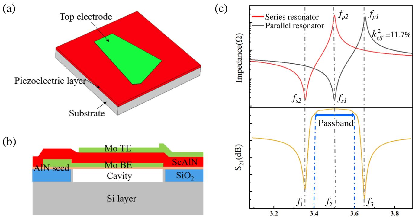
**Figure 1.** Structures of FBAR and characteristics of filters. (a) Schematic drawing of a typical FBAR. (b) The cross-sectional view of FBAR. (c) Working principle of filter based on FBARs in the circuits model.
