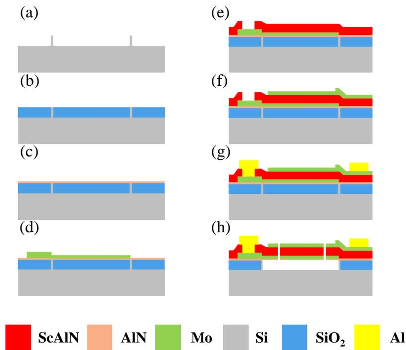
**Figure 2.** Fabrication of the Sc<sub>0.2</sub>Al<sub>0.8</sub>N-based FBARs. (a) The film structure of FBAR. (b) Forming separation walls. (c) SiO<sub>2</sub> deposition and chemical mechanical polishing. (d) Seed layer deposition. (e) Bottom Mo and Sc<sub>0.2</sub>Al<sub>0.8</sub>N layers were dual-deposited and then patterned. (f) Top Mo was dual-deposited and then patterned. (g) Al was deposited and then patterned. (h) Opening the release window and release.
