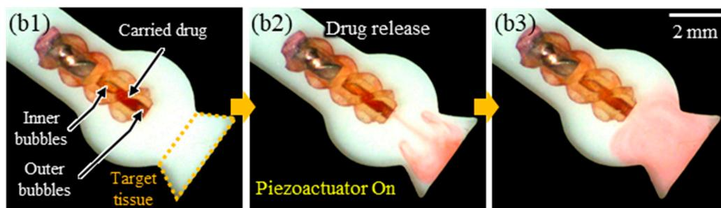
**Figure 11.** Sequential snapshots of the proposed targeted drug delivery technology: (a1–a3) magnetic actuation of a fabricated microrobot in a Y-shaped channel filled with water; (b1–b3) drug manipulation (carrying and releasing) by acoustically controlling bubbles embedded in the microrobot.
