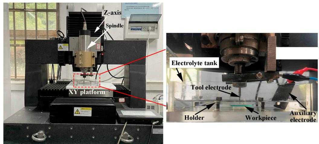
**Figure 1.** Diagram of the experimental setup.
