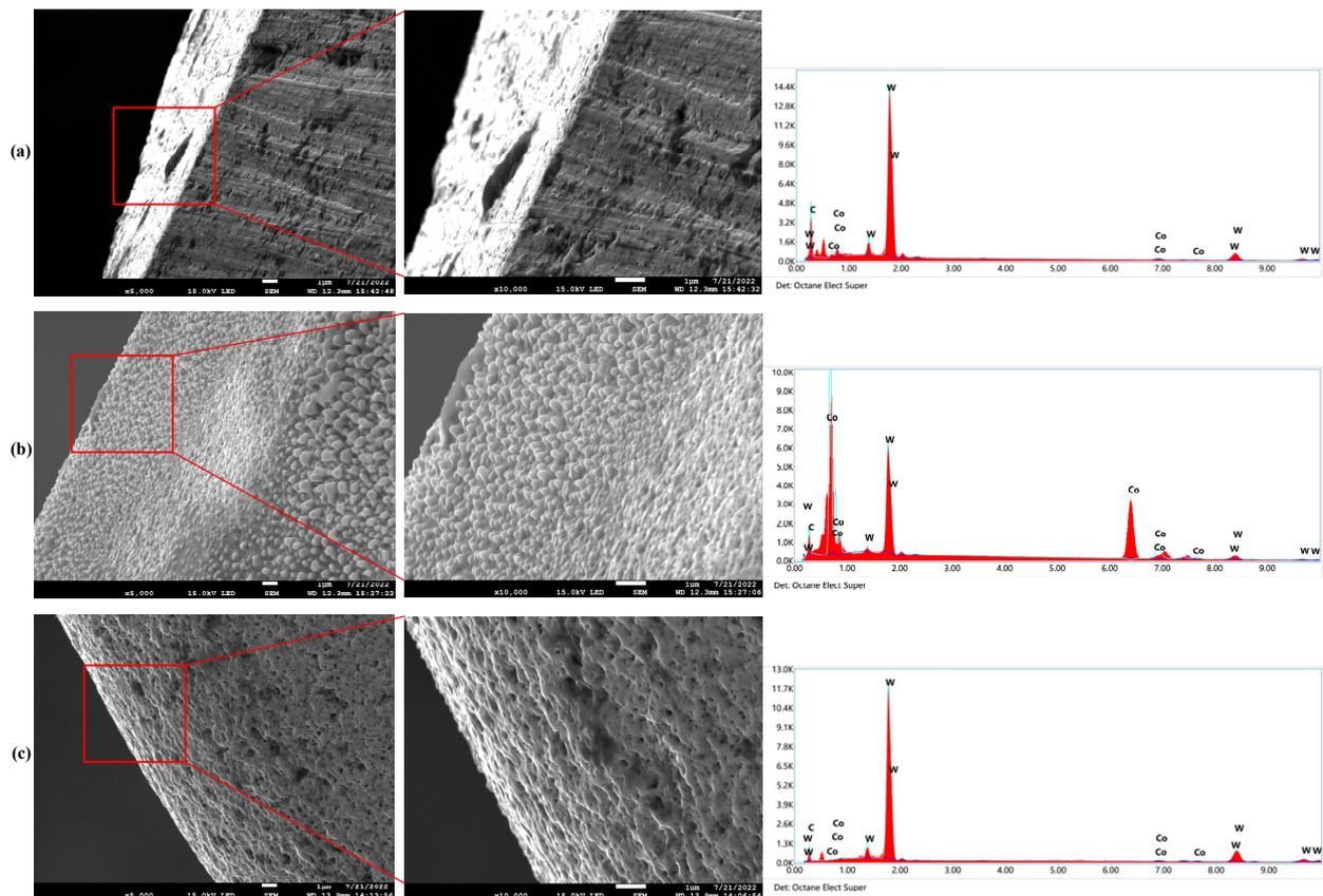
**Figure 11.** The EDS results of the cutting edge of the tool electrodes before and after machining in two different electrolytes. (a) Before machining. (b) After machining in conventional electrolyte. (c) After machining in graphite-powder-mixed electrolyte.
