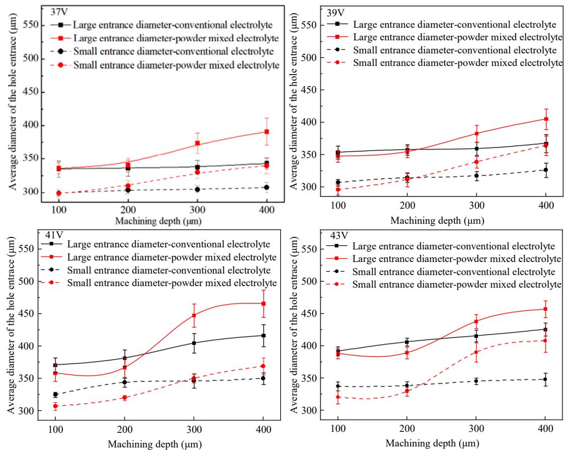
**Figure 6.** Variation of the average diameter of the hole entrance with machining depth.
