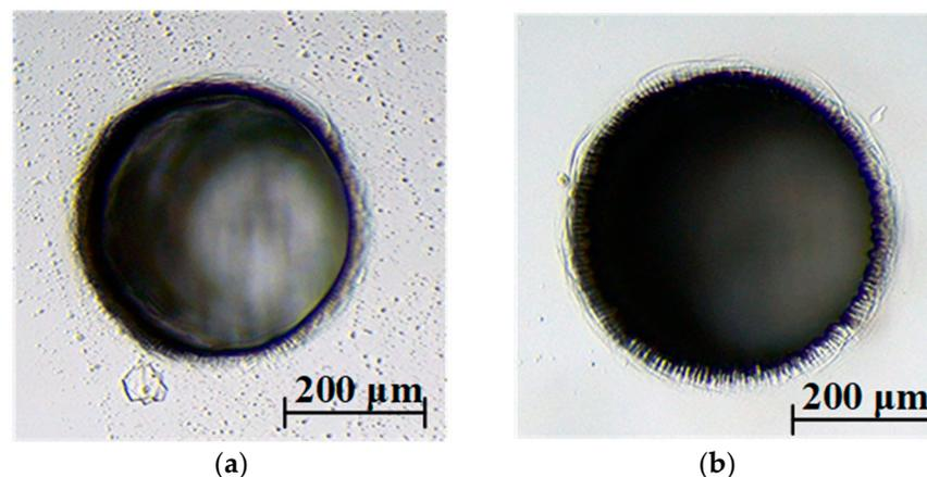
**Figure 5.** Microholes with a depth of  $400\ \mu\text{m}$  machined in different electrolytes. (a) Conventional electrolyte. (b) Graphite-powder-mixed electrolyte.
