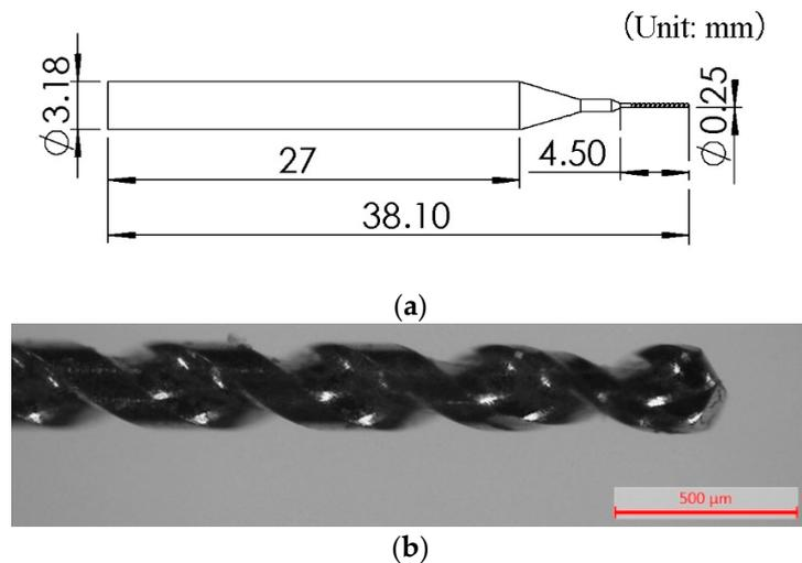
**Figure 2.** The dimension and shape of the microdrill bit. (a) The dimension of the microdrill bit. (b) The working part of the microdrill bit.
