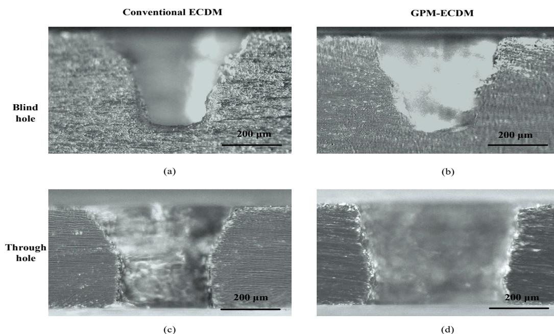
**Figure 9.** Cross sections of 400  $\mu\text{m}$  depth blind and through holes machined at 37 V. (a) Blind hole machined in the conventional electrolyte. (b) Blind hole machined in the graphite powder mixed electrolyte. (c) Through hole machined in the conventional electrolyte. (d) Through hole machined in the graphite powder mixed electrolyte.
