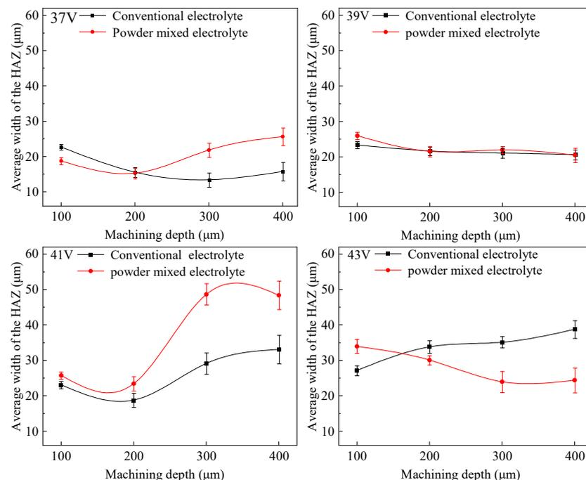
**Figure 7.** Variation of HAZ width with machining depth.
