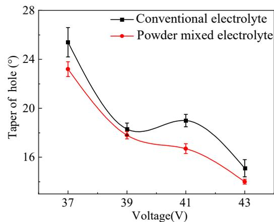
**Figure 8.** Variation of the hole taper with machining voltage in different electrolytes.
