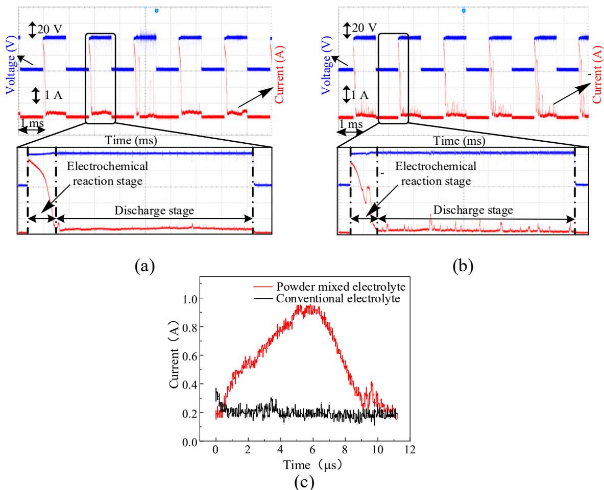
**Figure 3.** The voltage and current signals in different electrolytes at the voltage of 41 V. (a) The conventional electrolyte. (b) The graphite-powder-mixed electrolyte. (c) Comparison between the small pulse current waveform and the conventional electrochemical discharge current waveform.
