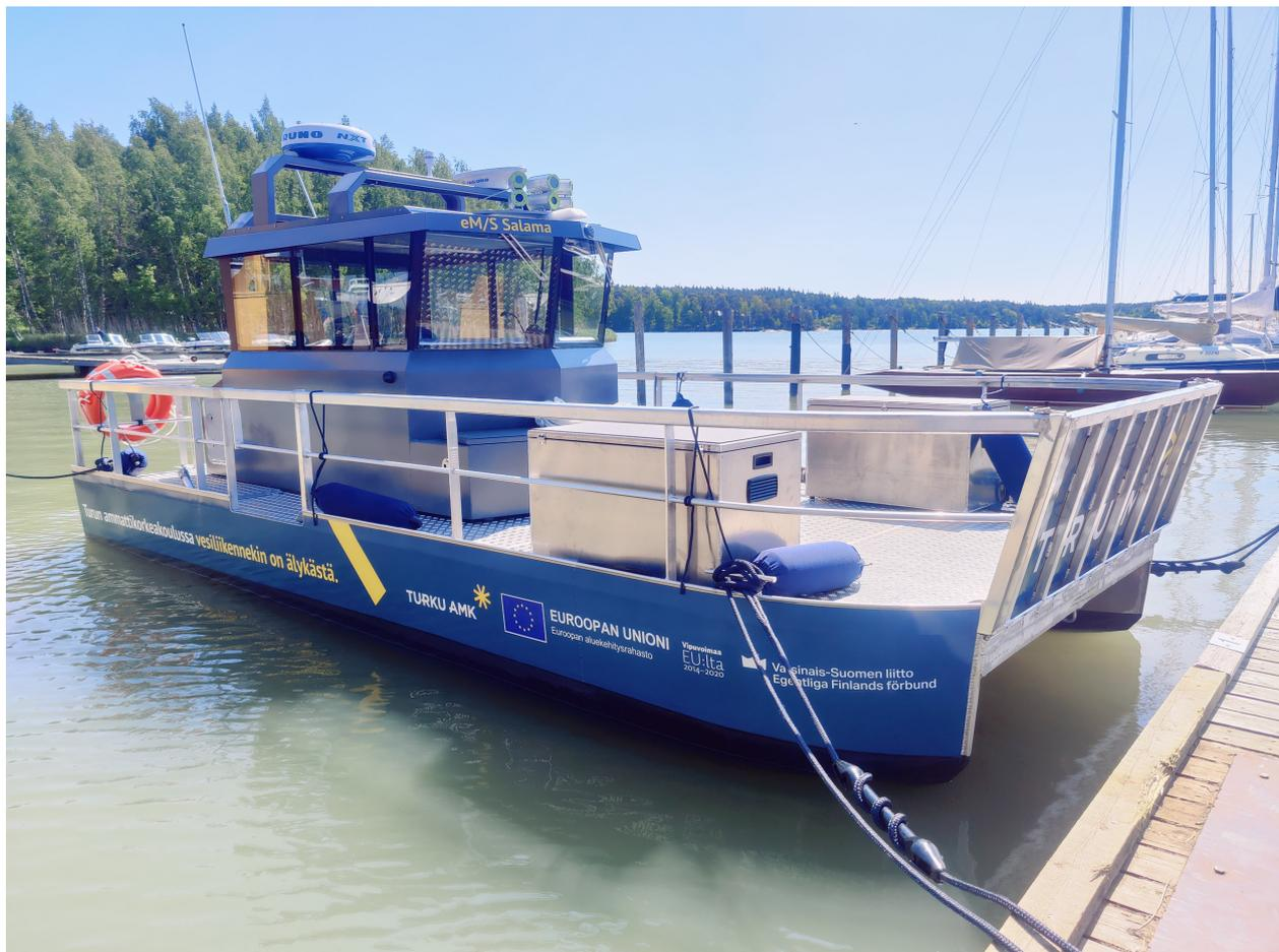
**Figure 2.** Unmanned Surface Vessel eM/S Salama.
