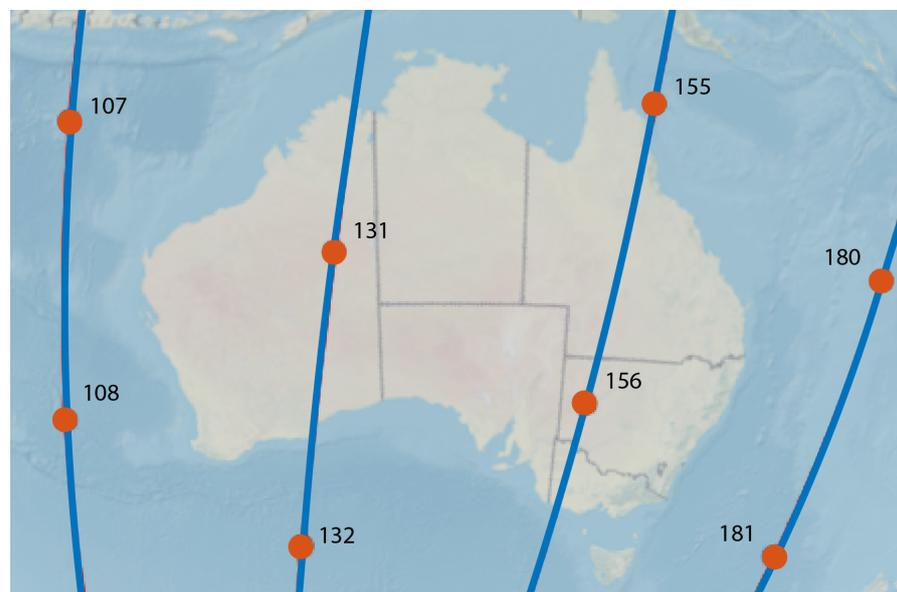
**Figure 2.** Example of satellite constellation orbits using Walker-star pattern with 12 orbital planes and 24 satellites distributed equally on a single plane.
