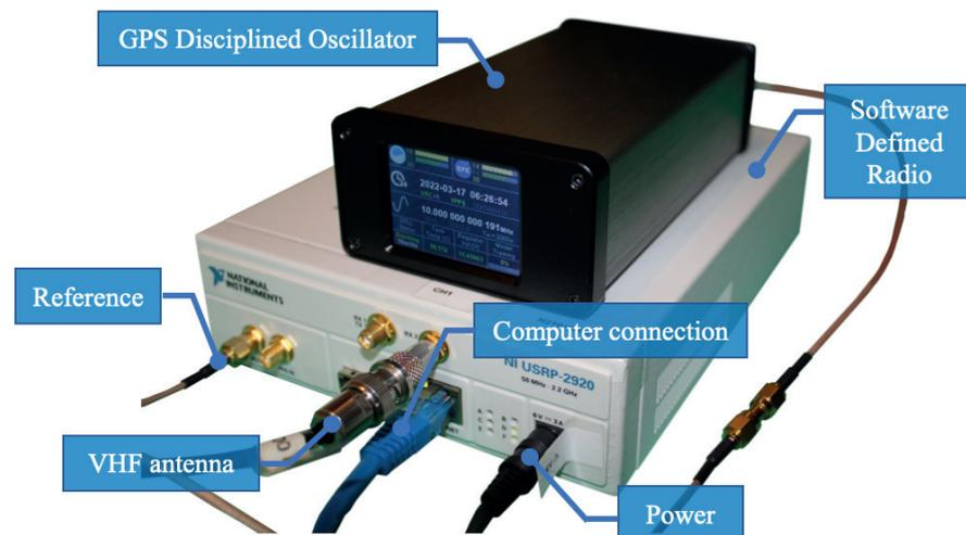
**Figure 10.** The connection between the Software-Defined Radio (National Instruments (NI) Universal Software Radio Peripheral (USRP) 2950) and the GPS-disciplined oscillator.
