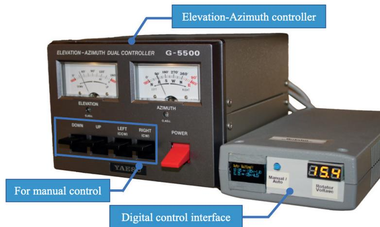
Figure 7. Satellite tracking antenna with digital control interface and elevation–azimuth controller connected to the antenna’s rotator.
