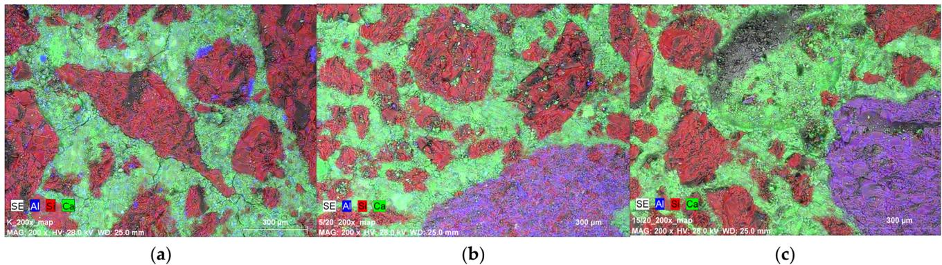
**Figure 7.** Microstructure of cement mortars with visible distribution of dominant chemical elements in this area at 200× magnification: (a) control mortar, (b) mortar containing 5% waste and (c) mortar containing 15% waste.
