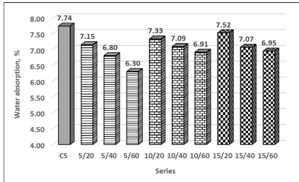
**Figure 5.** Water absorption of investigated cement mortar modified with waste polyamide 6.
