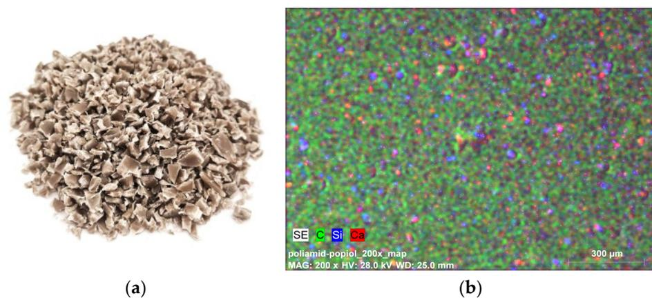
**Figure 1.** Waste polyamide 6 modified with 15% fly ash (a) and a microscope photo at 400× magnification with the dominant elements in this area (b).
