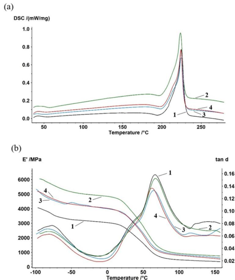
**Figure 2.** DSC (a) and DMTA (b) thermograms for fly ash-modified polyamide: 1—PA, 2—A + 5% biomass fly ash, 3—PA + 10% biomass fly ash, 4—PA + 15% biomass fly ash.
