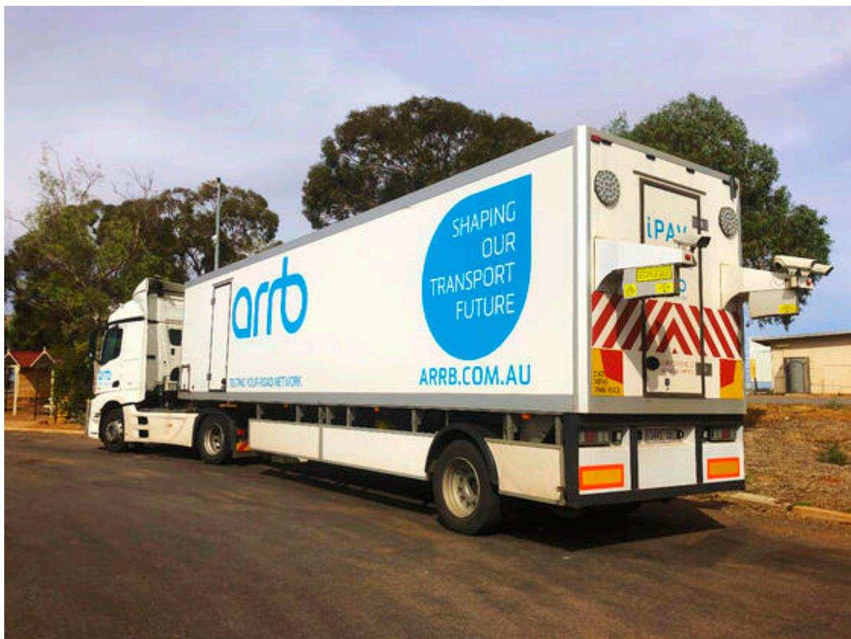
**Figure 2.** iPAVe used to collect pavement condition data in South Carolina (source: <https://www.arrb.com.au/ipave> accessed on 13 July 2022).
