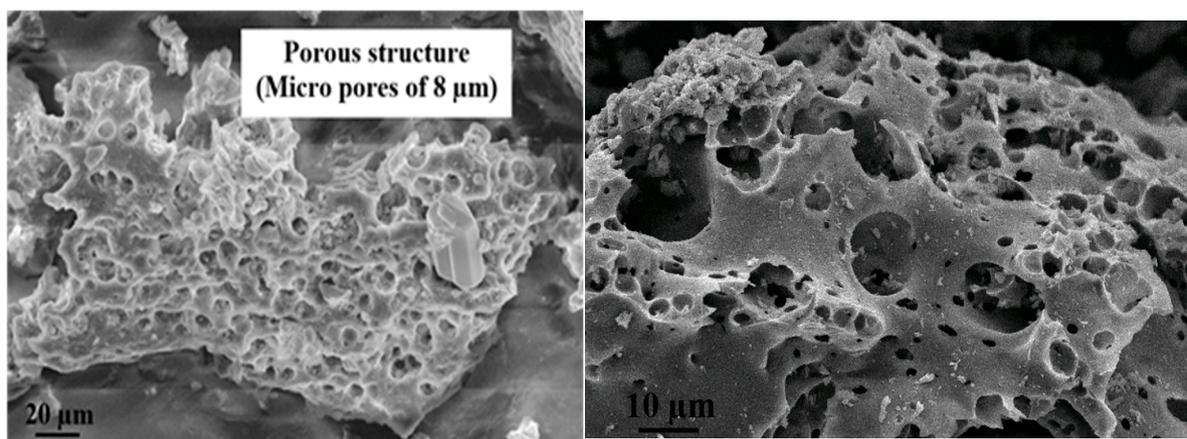
**Figure 2.** Porous structure of coal bottom ash.
