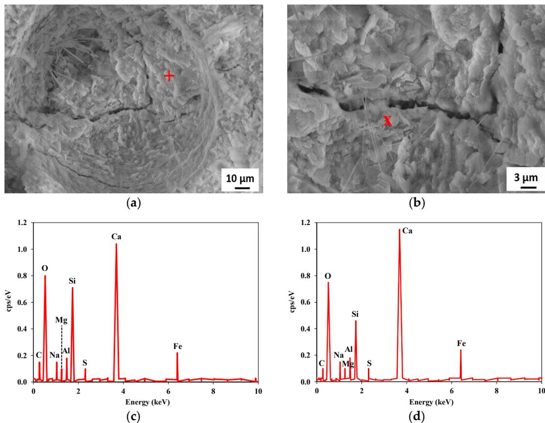
**Figure 13.** SEM and EDX analyses of control specimen without CBA at 56 days immersion in NaOH solution. (a,b) Cracking in control specimens subjected to ASR conditions, (c) EDX at (+), and (d) EDX at (x).
