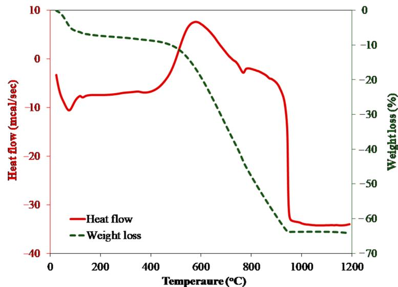
Figure 5. Thermal analysis of untreated coal bottom ash.
