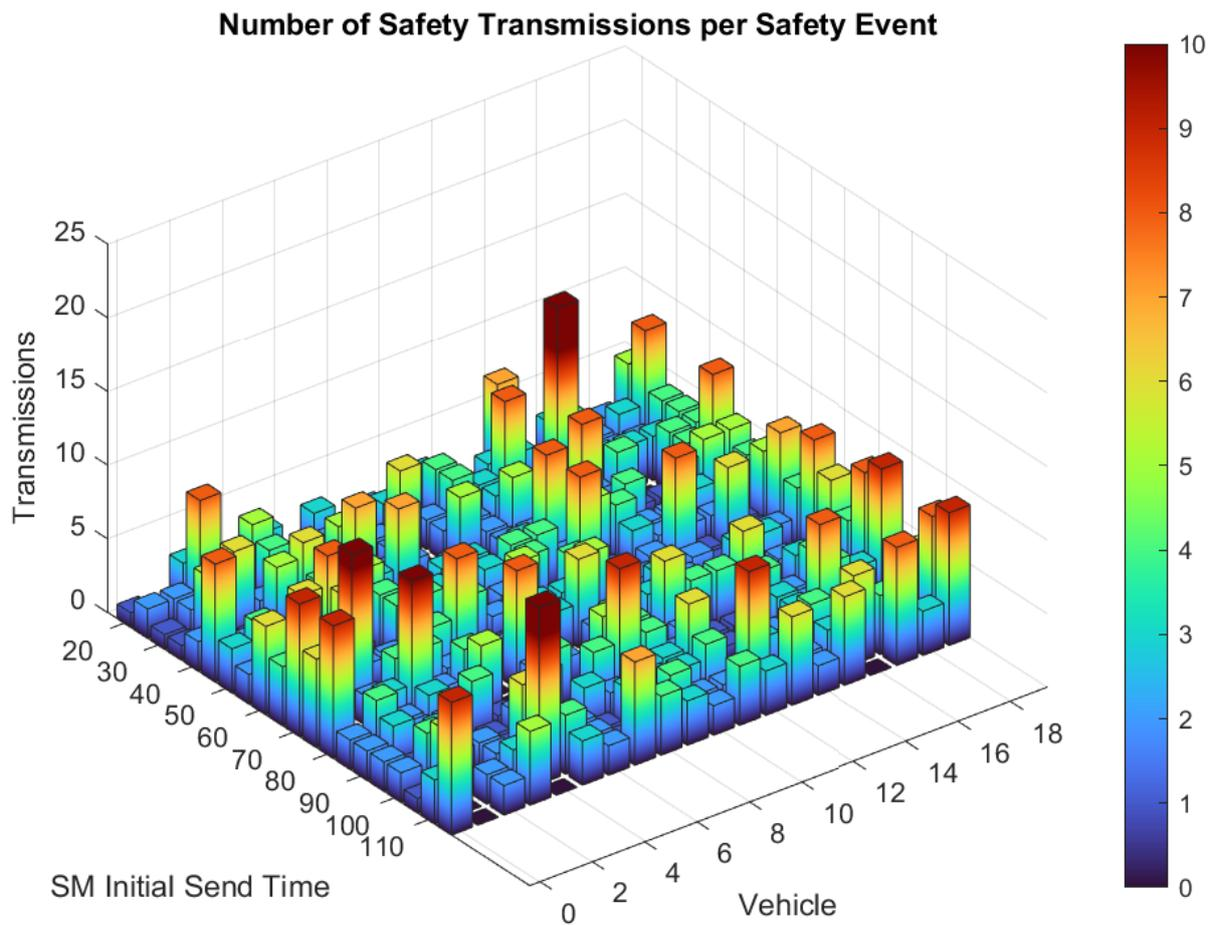
Figure 14. Far spacing, standard delays. Number of SM transmissions per event for every vehicle given the SM transmission time.
