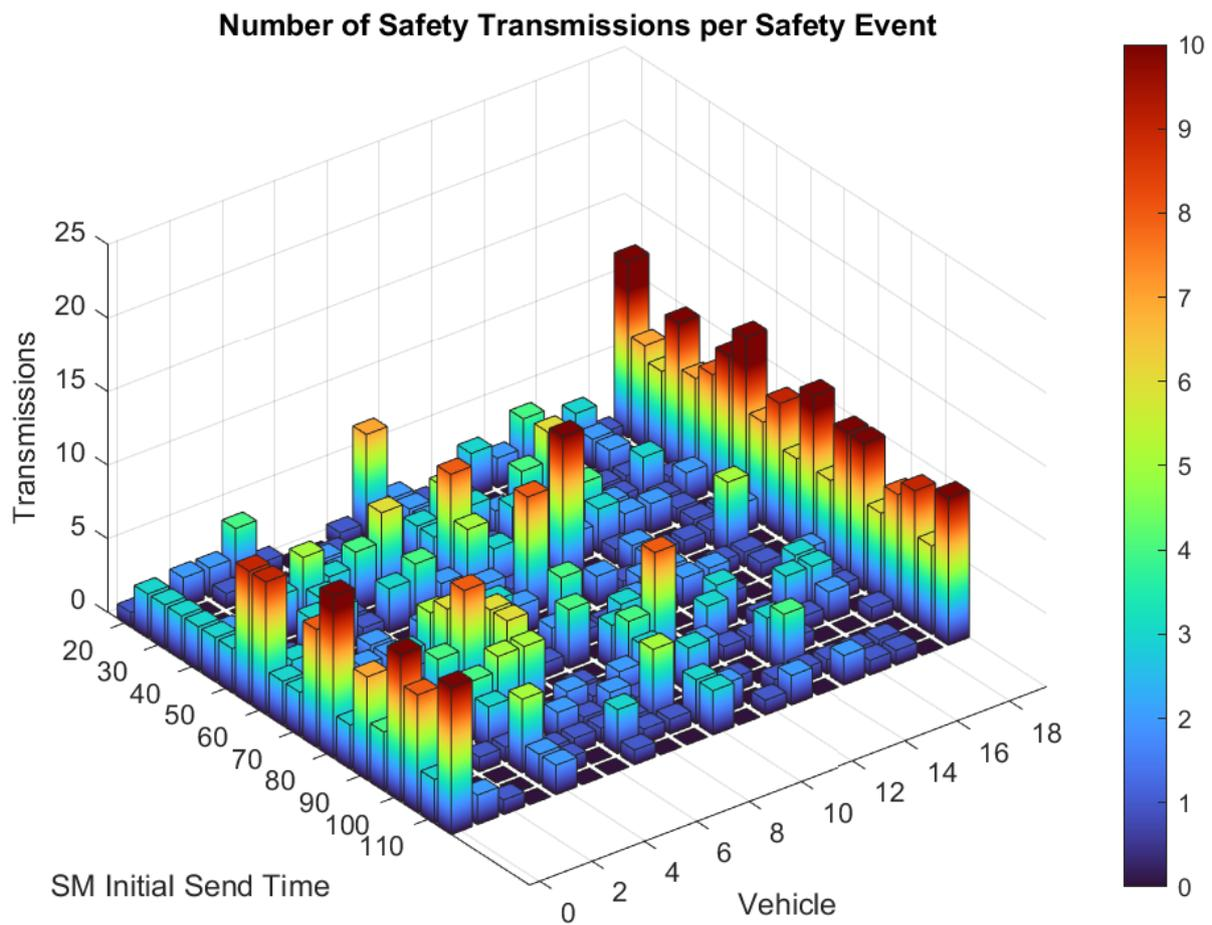
**Figure 8.** Close spacing, standard delays. Number of SM transmissions per event for every vehicle given the SM transmission time.
