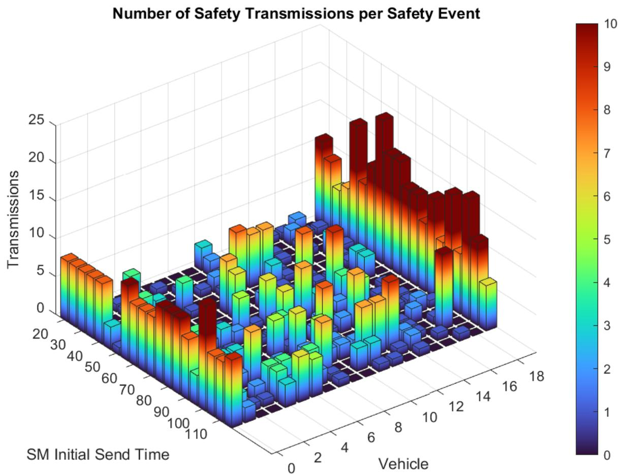
**Figure 10.** Close spacing, doubled delays. Number of SM transmissions per event for every vehicle given the SM transmission time.
