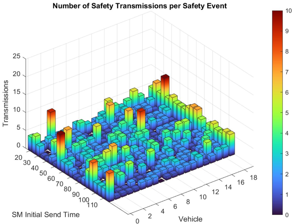
**Figure 2.** Standard spacing, standard delays. Number of SM transmissions per event for every vehicle given the SM transmission time.
