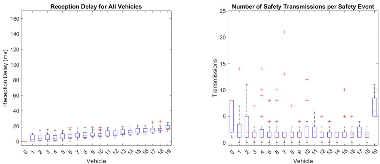
**Figure 3.** Standard spacing, doubled delays. (Left): SM reception delay for every vehicle. (Right): Number of SM transmissions for every vehicle.
