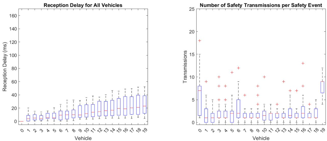
Figure 25. Far-to-close spacing, doubled delay randomness. (Left): SM reception delay for every vehicle. (Right): Number of SM transmissions for every vehicle.
