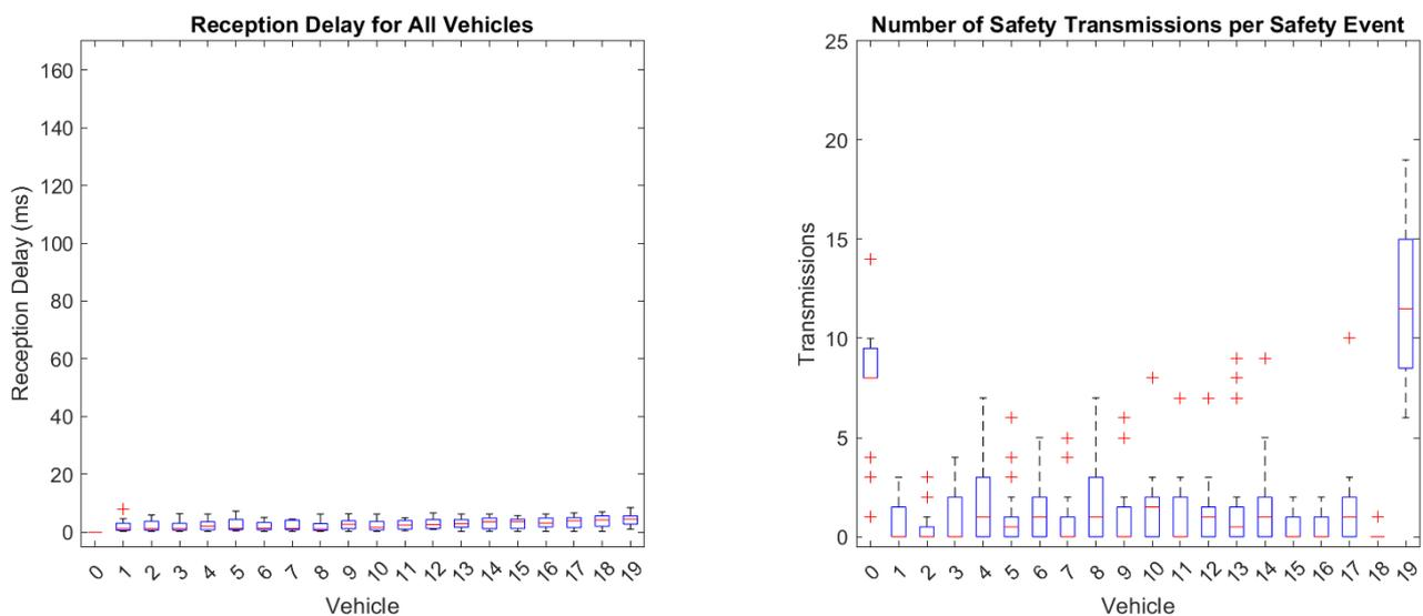
**Figure 9.** Close spacing, doubled delays. (Left): SM reception delay for every vehicle. (Right): Number of SM transmissions for every vehicle.
