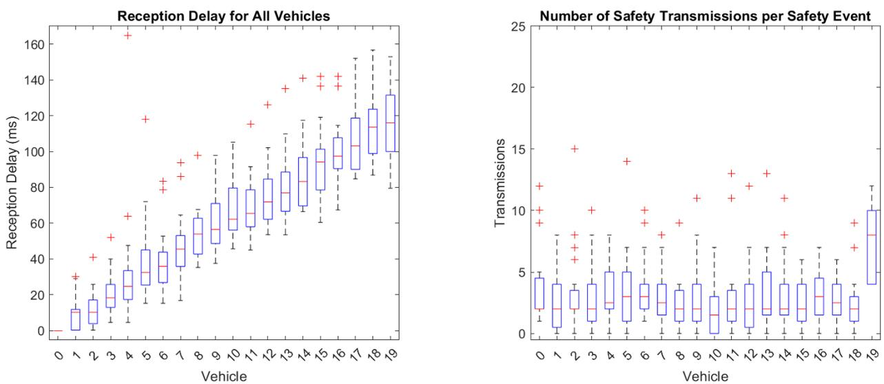
Figure 15. Far spacing, doubled delays. (Left): SM reception delay for every vehicle. (Right): Number of SM transmissions for every vehicle.
