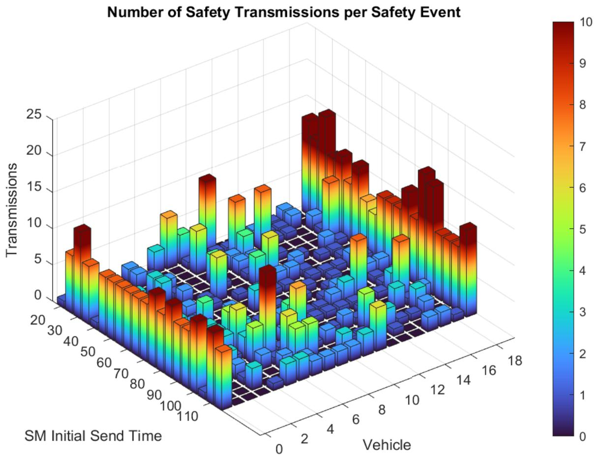
**Figure 12.** Close spacing, doubled delay randomness. Number of SM transmissions per event for every vehicle given the SM transmission time.
