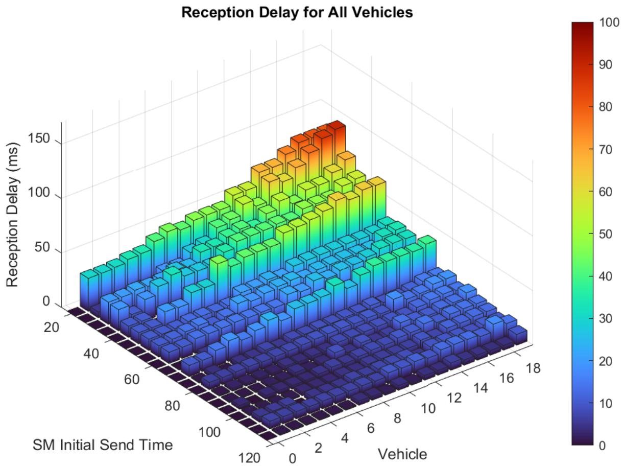
Figure 24. Far-to-close spacing, doubled delays. SM reception delay for every vehicle and SM event.
