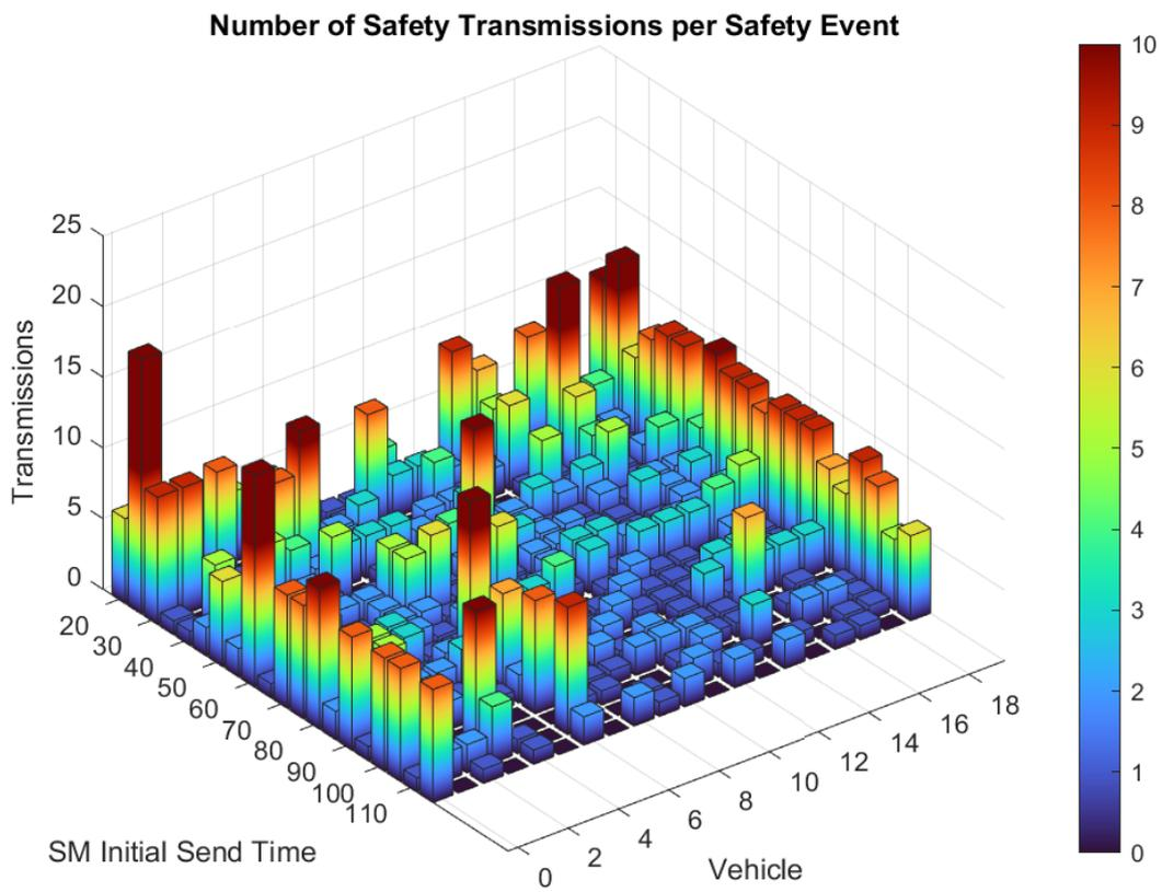
**Figure 26.** Far-to-close spacing, doubled delay randomness. Number of SM transmissions per event for every vehicle given the SM transmission time.
