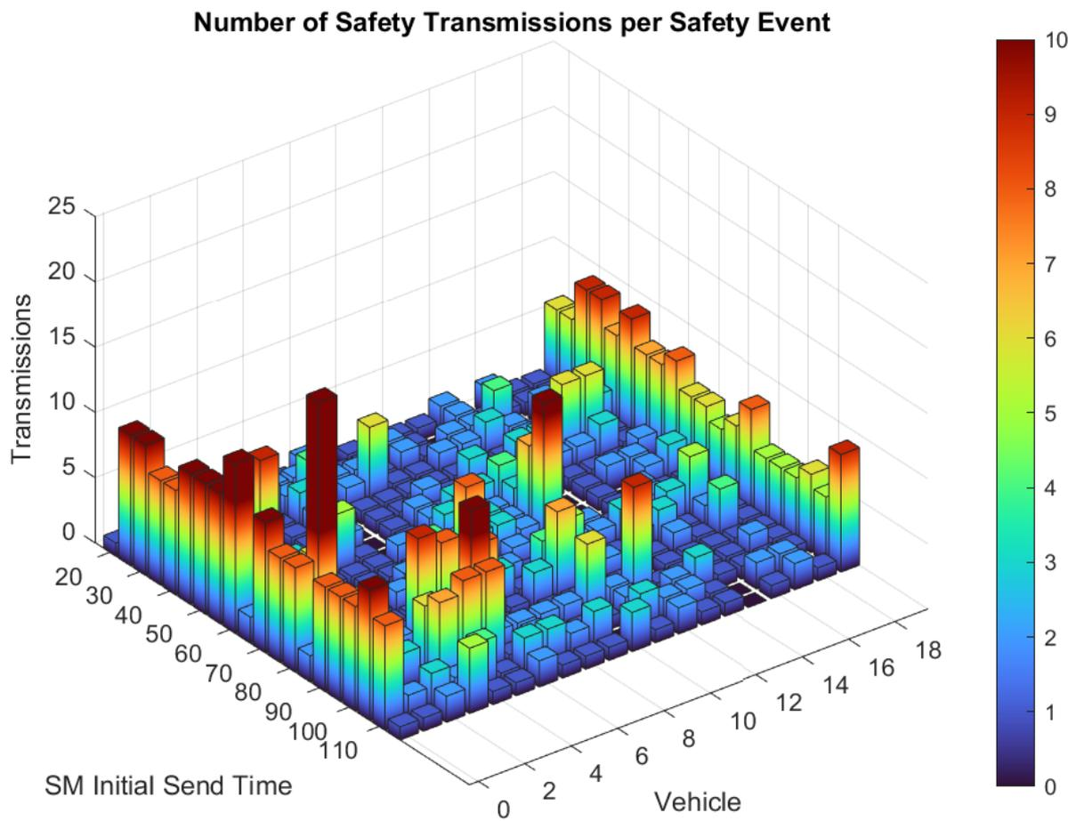
**Figure 6.** Standard spacing, doubled delay randomness. Number of SM transmissions per event for every vehicle given the SM transmission time.
