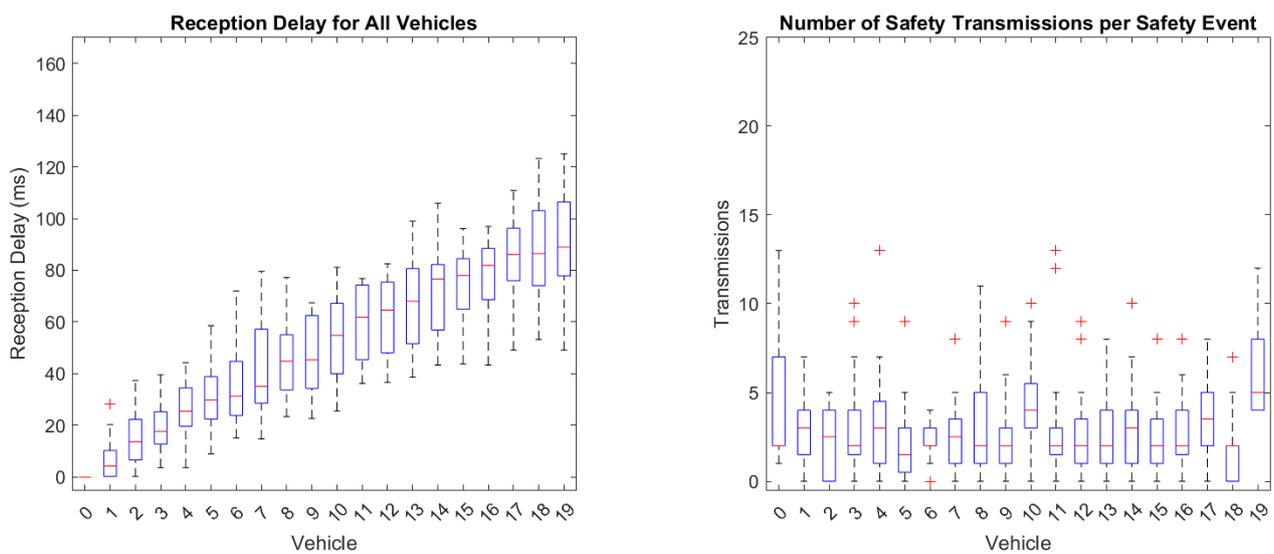
**Figure 17.** Far spacing, doubled delay randomness. (Left): SM reception delay for every vehicle. (Right): Number of SM transmissions for every vehicle.
