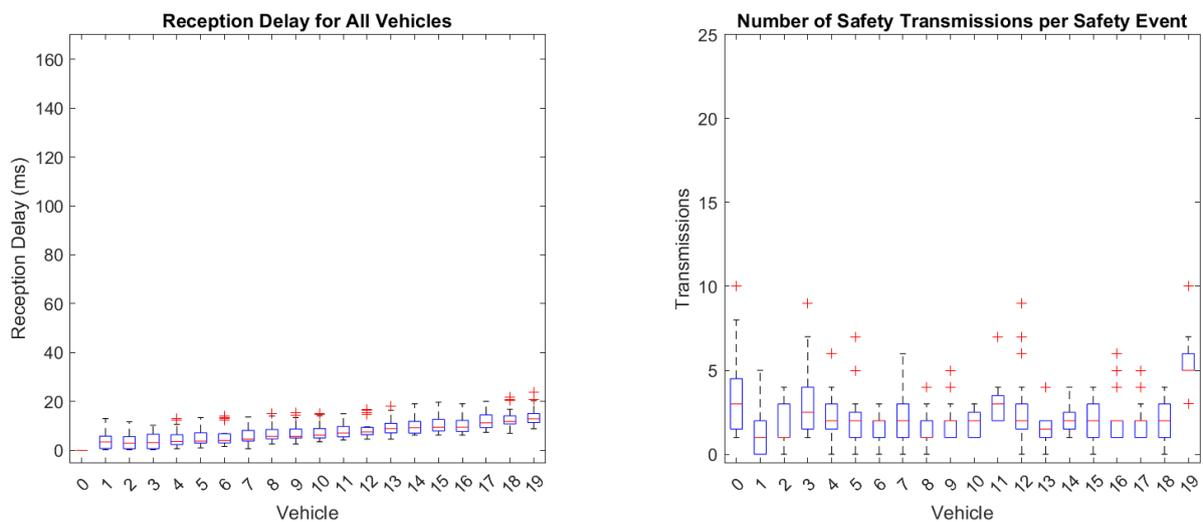
**Figure 1.** Standard spacing, standard delays. **(Left):** SM reception delay for every vehicle. **(Right):** Number of SM transmissions for every vehicle.
