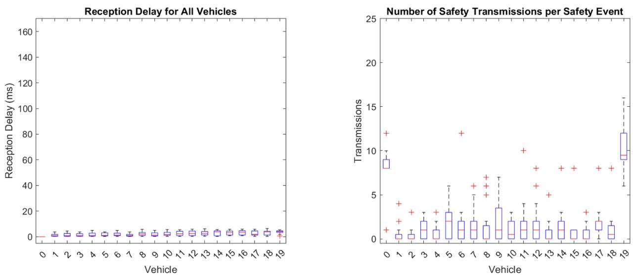
**Figure 11.** Close spacing, doubled delay randomness. **(Left):** SM reception delay for every vehicle. **(Right):** Number of SM transmissions for every vehicle.
