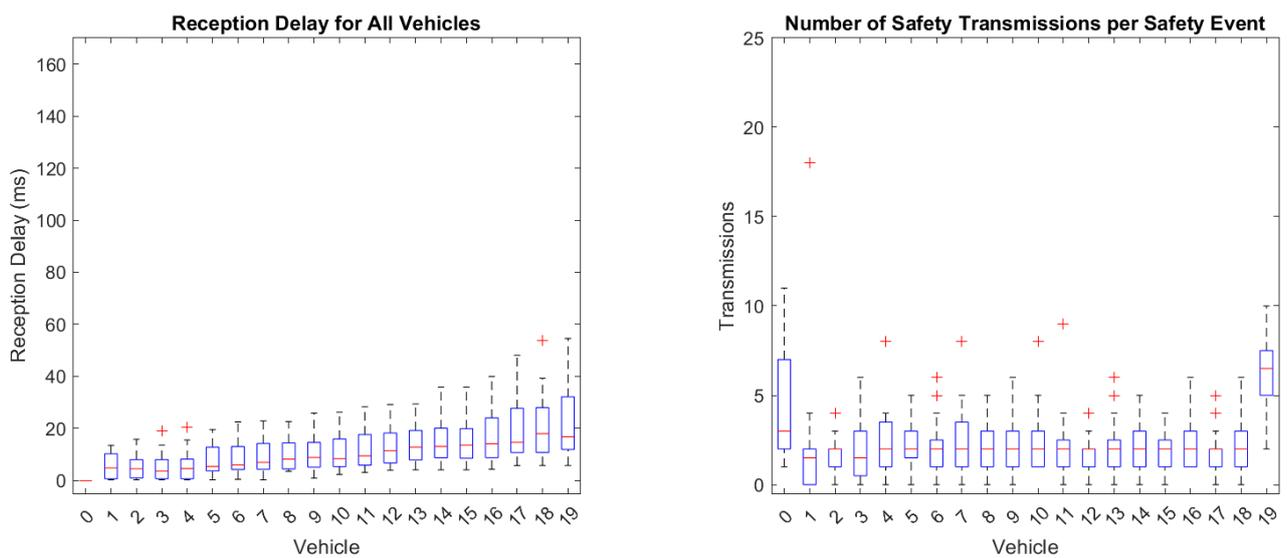
**Figure 19.** Far-to-close spacing, standard delays. (Left): SM reception delay for every vehicle. (Right): Number of SM transmissions for every vehicle.
