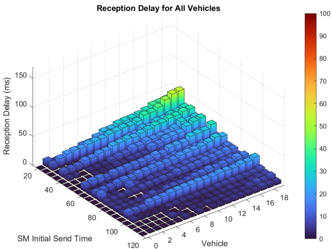
**Figure 21.** Far-to-close spacing, standard delays. SM reception delay for every vehicle and SM event.
