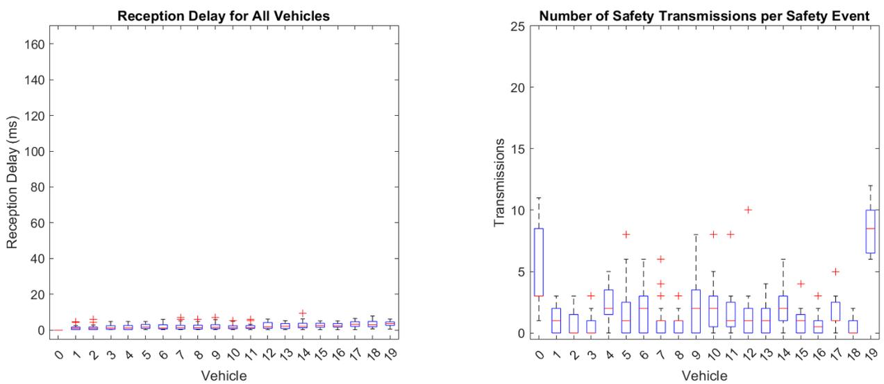
**Figure 7.** Close spacing, standard delays. (Left): SM reception delay for every vehicle. (Right): Number of SM transmissions for every vehicle.
