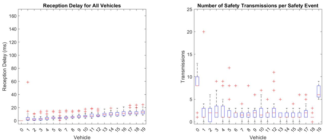
**Figure 5.** Standard spacing, doubled delay randomness. (Left): SM reception delay for every vehicle. (Right): Number of SM transmissions for every vehicle.
