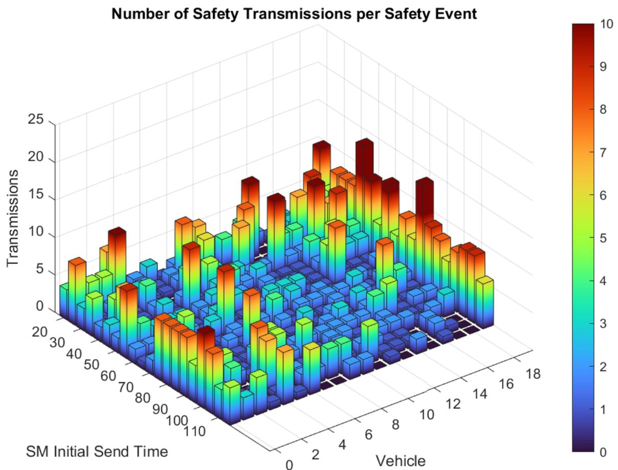
**Figure 23.** Far-to-close spacing, doubled delays. Number of SM transmissions per event for every vehicle given the SM transmission time.
