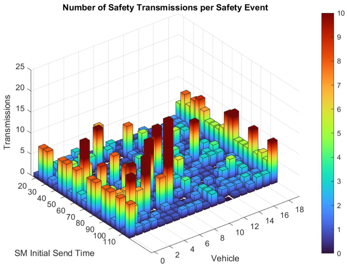
**Figure 4.** Standard spacing, doubled delays. Number of SM transmissions per event for every vehicle given the SM transmission time.
