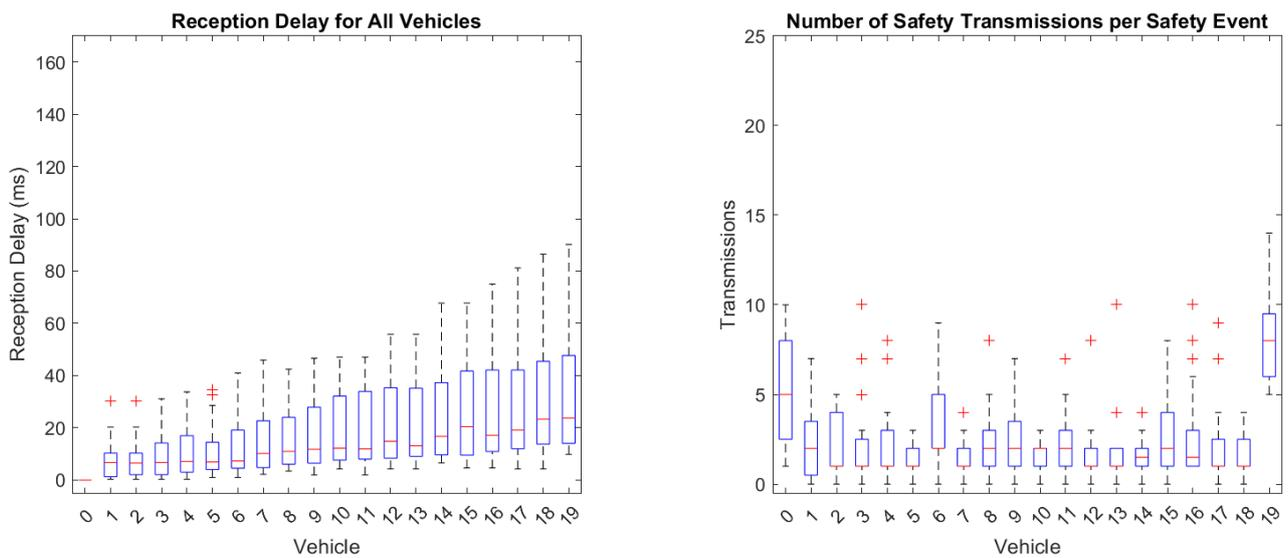
**Figure 22.** Far-to-close spacing, doubled delays. **(Left):** SM reception delay for every vehicle. **(Right):** Number of SM transmissions for every vehicle.
