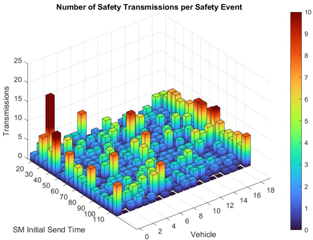
**Figure 20.** Far-to-close spacing, standard delays. Number of SM transmissions per event for every vehicle given the SM transmission time.
